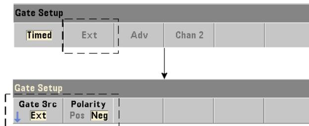
When using any external gate source the polarity of the gate signal and therefore, the duration of the gate, is set or changed with the command:
