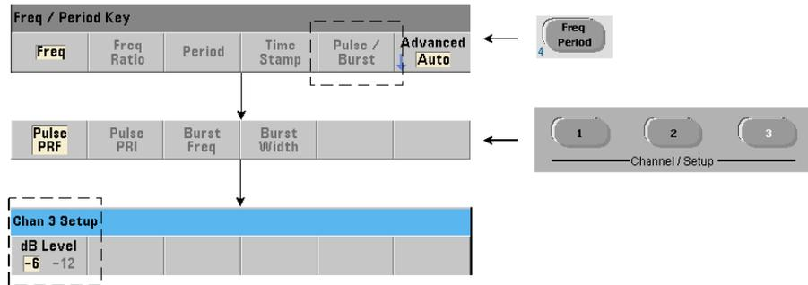
All 53230A burst measurements are relative to the pulse width. The 'on' portion of the pulse width is established by a -6 dB and -12 dB detector threshold. Figure 4-6 is an example of the thresholds relative to the peak amplitude of the burst signal.
