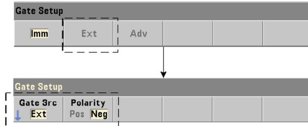
When using an external gate source, the polarity of the gate signal is changed with the command:
