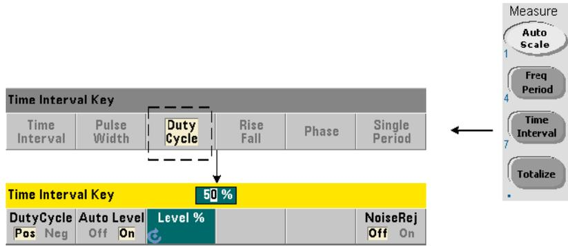
Positive and negative duty cycle measurements are the ratio of the positive or negative widths to the period of the signal (Figure 3-10).
