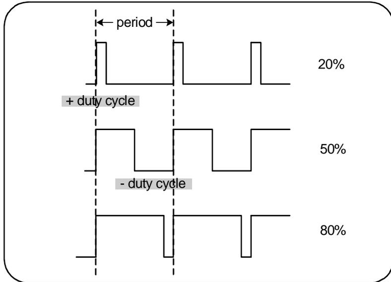
Figure 3-10. Positive and Negative Duty Cycle Measurements.
