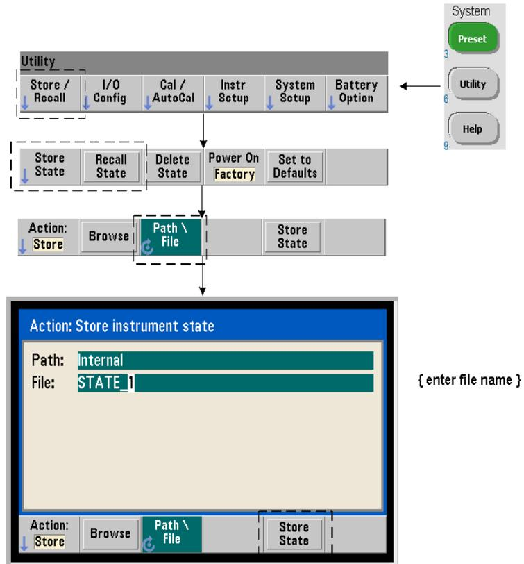
Instrument states can be stored in the instrument's internal flash memory or on a USB memory device and recalled later to restore a specific configuration (Figure 7-2).
