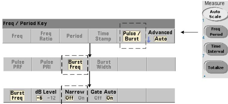
For carrier frequency measurements with ‘on durations’ (Figure 5-6) less than 10  $\mu$ s, narrow pulse mode must be set using the command:
