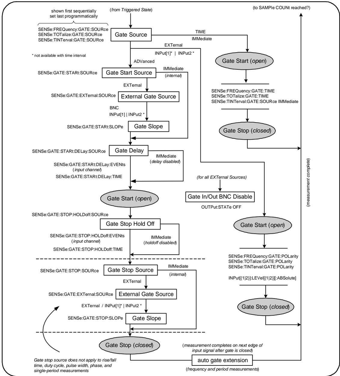
Figure 5-2 (cont'd). Trigger and Gate Cycle - Gating.
