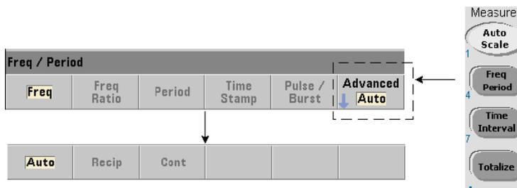
There are three measurement modes available for making **frequency**, **frequency ratio**, and **average period** measurements. The measurement mode is set using the command:
