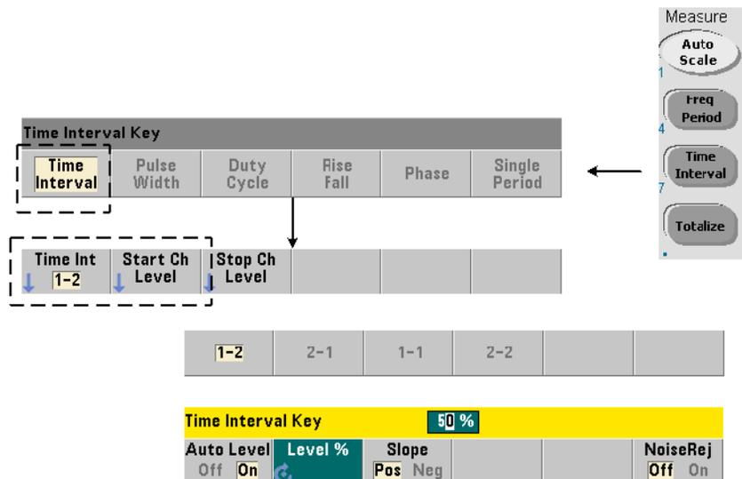
A time interval measurement is the difference between two events, or edges, on different waveforms or on the same waveform. A typical two-channel time interval measurement is shown in Figure 3-6.
