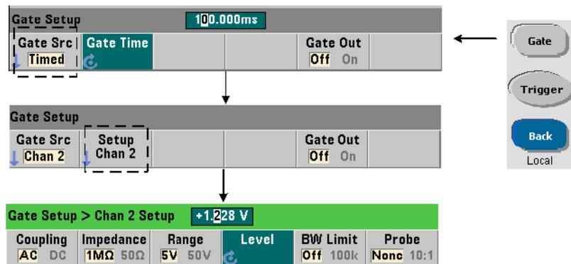
For external sources INPut[1] and INPut2 (Chan 1 and Chan 2 softkeys), a **fixed** input threshold voltage must be specified in addition to the gate signal polarity. This is done using the command:
