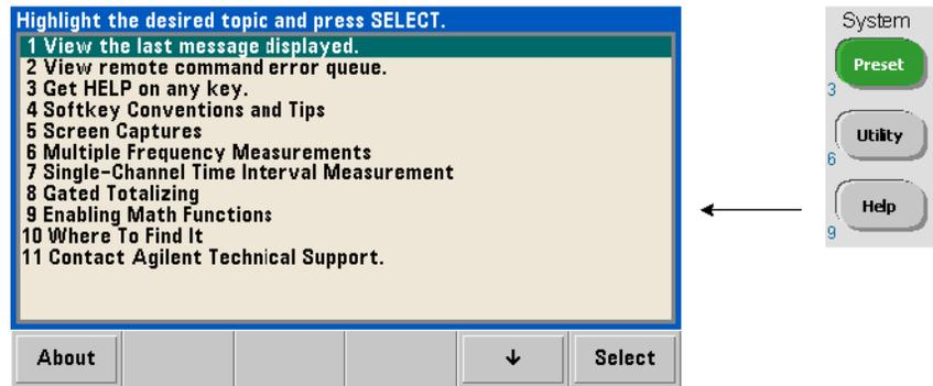
Instrument help is available by pressing and holding any front panel key or softkey. Pressing the Help key enables you to select additional help topics including front panel measurement examples.
