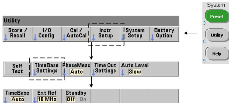
53220A and 53230A measurements are based on a reference oscillator - also referred to as an internal/external clock or time base. A valid reference oscillator signal must be present for measurements to occur.
