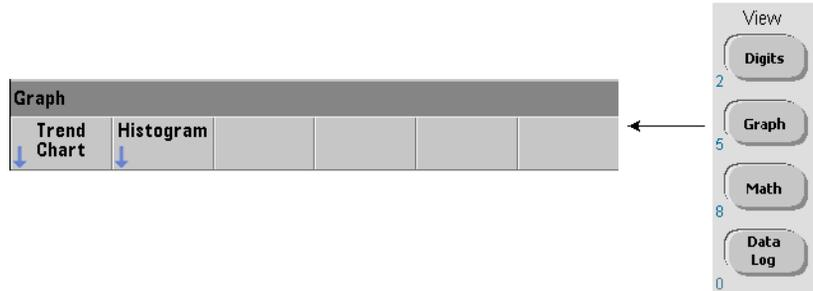
At power-on or following a reset (\*RST) or instrument preset (Preset), numeric data is displayed. The display can be changed to a trend chart by changing the display mode using the command:
