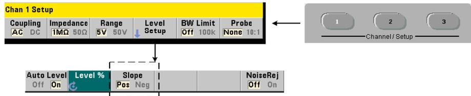
The slope (edge) of the input signal on which the threshold level occurs is specified with the command:
