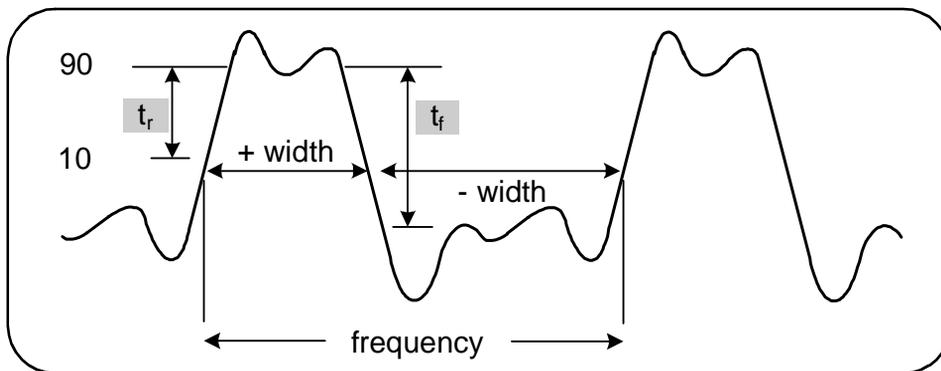
Figure 3-8. Rise Time and Fall Time Measurements.
