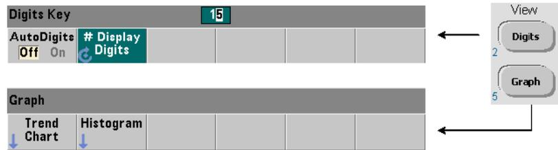
With AutoDigits On, the number of digits displayed is automatically set based on gate time, measurement mode (AUTO, CONTinuous, RECiprocal - Chapter 3), and resolution enhancement. When Off, the number of digits is set with the rotary knob or [Shift]ed numeric keys. See “Resolution and Gate Time” in Chapter 5 for more information when AutoDigits On is set.
