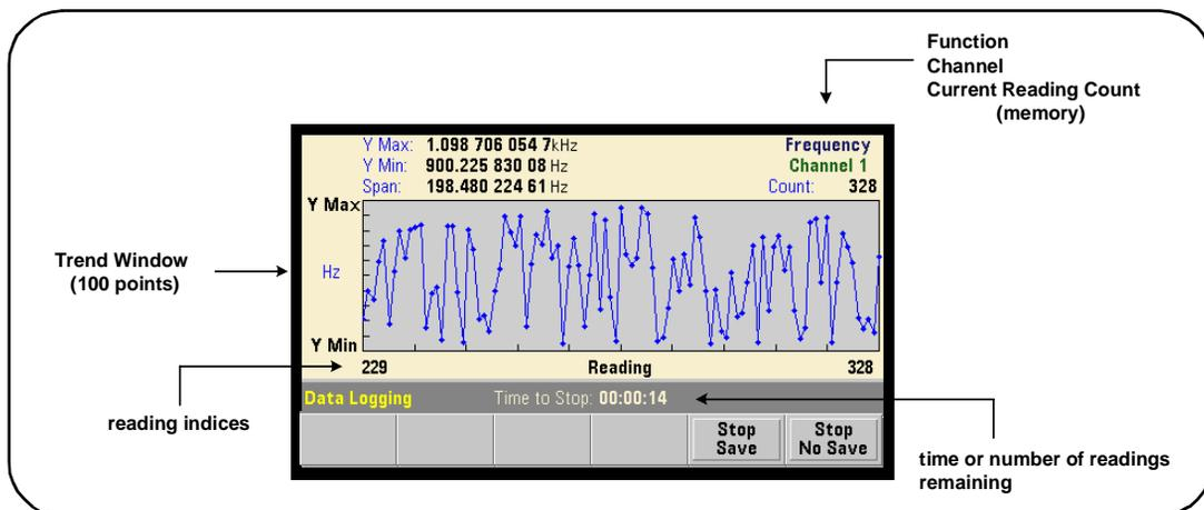
**Figure 6-12. Trend Chart Display During Data Logging.**
