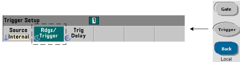
The trigger count multiplied by the sample count ( $\text{TRIG:COUN} \times \text{SAMP:COUN}$ ) determines the number of readings taken before the counter returns to the *idle* state. The sample count is set with the command:
