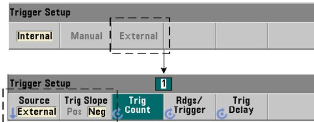
When the system trigger source is set to `EXTErnal`, the triggering slope (edge) of the signal is set with the command:
