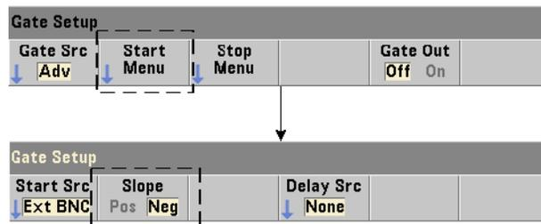
When using the external gate sources listed, the polarity of the start gate signal is set (changed) with the command:
