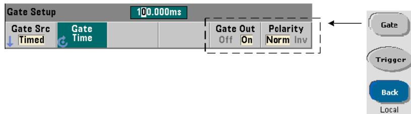
For timing and synchronization with other instruments gate signals from sources Time (internal), IMMEDIATE (internal), and INPUT[1]/INPUT2 (Chan 1 and Chan 2 softkeys) can be routed to the rear panel 'Gate In/ Out' connector and assigned a polarity using the commands:
