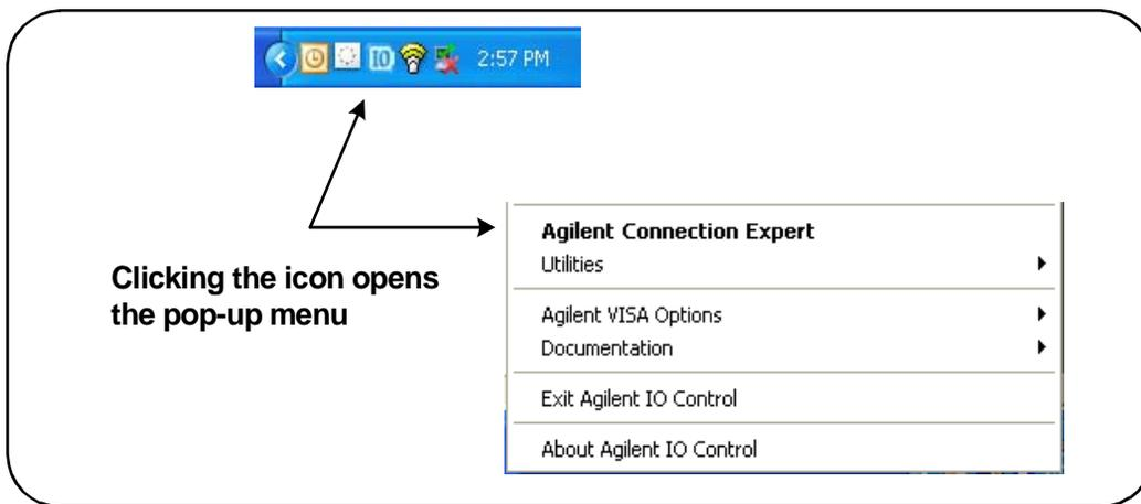
**Figure 2-3. Starting Agilent Connection Expert.**
