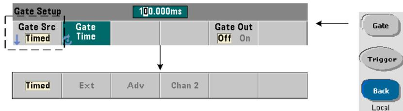
Gate sources **EXTernal**, **INPut[1]**, and **INPut2** are external sources. **EXTernal** is the counter's rear panel 'Gate In/Out' BNC, and **INPut[1]** / **INPut2** (represented by softkeys Chan 1 and Chan 2) are the counter's channel 1 and channel 2 inputs.
