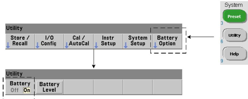
With Battery Option 300 installed and **enabled**, the 53220A/53230A counter can be operated using battery power for up to three hours.
