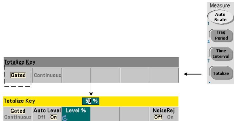
Gated (timed) totalizing measurements count events (edges) that occur on the channel over a specified period.
