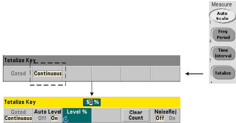
Continuous totalizing measurements count events (edges) that occur on the input channel.
