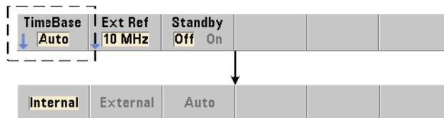
The reference oscillator (time base) is either the counter’s internal oscillator or the internal oscillator tuned to an external reference. The source commands are:
