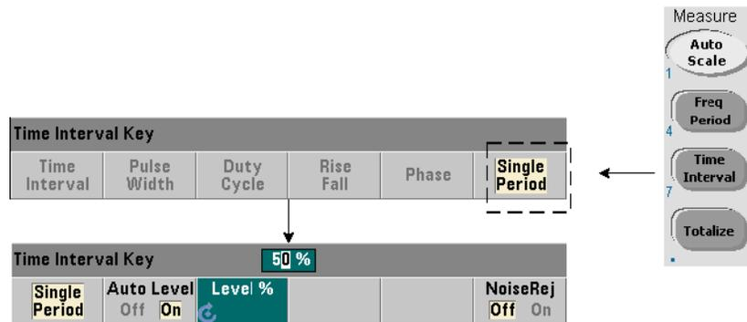
A form of time interval measurement - the single-period measurement, is based on a **single** waveform cycle. Single-period measurements provide measurement of “single-shot” or one cycle events; and allow analysis of signal characteristics (e.g. jitter) that would otherwise be averaged out with standard (averaging) period measurements.
