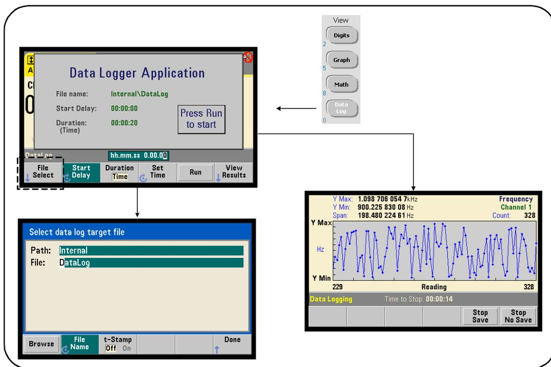
Figure 6-11. Starting the Counter Data Logger.
