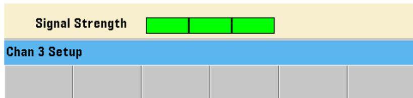
The relative signal strength on channel 3 Option 106 or 115 (6 GHz or 15 GHz microwave input) is displayed on the counter and can also be measured with the command:
