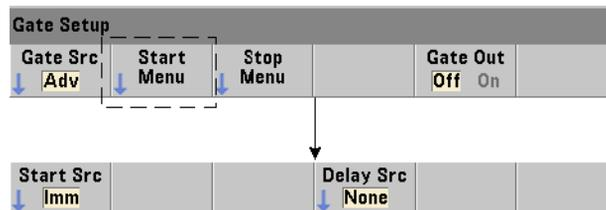
The specific command which sets the gate start (open) source is:
