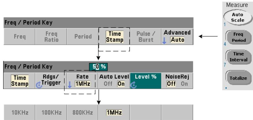
Time stamp measurements record events (edges) as they occur on the counter input channels. An example of time stamp measurements between the edges of an input waveform is shown in Figure 3-5. (Time stamp measurements are available with the **53230A only**.)
