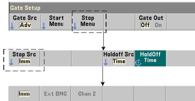
The gate stop source determines when the measurement gate is closed **following** the stop hold off.
