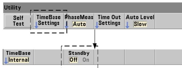
Standby power to maintain the operating temperature of the counter's internal OCXO reference oscillator (Option 010) is provided by the the line voltage or from Battery Option 300. Standby power is enabled and disabled using the command:
