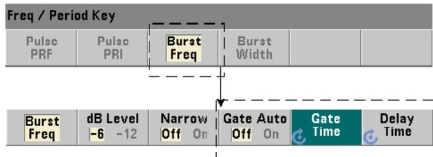
Gate control for measuring the carrier frequency can occur automatically during the measurement or be controlled manually as shown in Figure 5-7.
