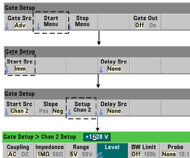
For external sources INPut[1] and INPut2 (Chan 1 and Chan 2 softkeys), a **fixed** input threshold voltage must also be specified in addition to the gate signal slope. This is done using the command:
