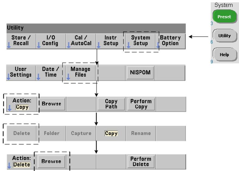
Folders and Files are deleted using the front panel as follows:
