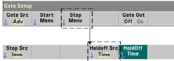
The gate stop holdoff source and its parameters are set with the commands:
