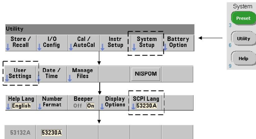
If the 53220A/53230A is sometimes used in 53132A SCPI language (emulation) mode, the instrument must be returned to its original (53220A/53230A) mode before the firmware can be updated.
