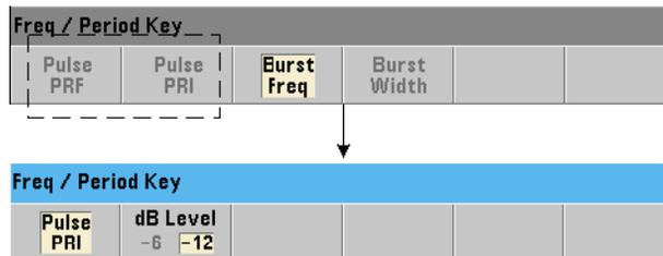
The commands used to measure the pulse repetition interval (PRI) and pulse repetition frequency (PRF) (Figure 3-13) of a burst signal are:
