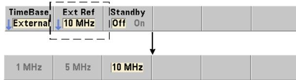
When the reference oscillator source is EXTERNAL as set by either `SENSe:ROSCillator:SOURce` or `SENSe:ROSCillator:SOURce:AUTO`, the lock frequency of the external signal (to which the internal oscillator is tuned) **must** be indicated using the command:
