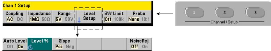
The threshold level is the trigger (input) level at which the counter begins the signal count (i.e. measurement). This level is the center of the hysteresis band - the band which represents counter sensitivity. For a count to occur, the signal must cross the upper and lower limits of the band in opposite directions (polarities). Figure 4-4 identifies these characteristics and conditions of the input signal. The dynamic range of the input signal is indicated on the front panel.
