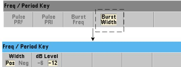
The commands used to measure the positive (on) width and negative (off) width of a burst pulse (Figure 3-13) are:
