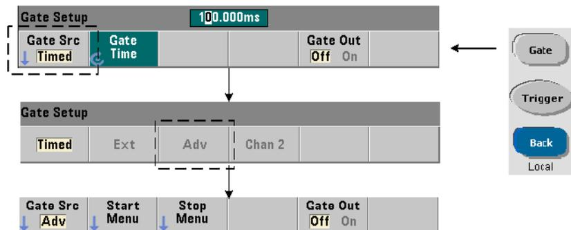
Setting the gate source to ADVanced during configuration of frequency, totalizing, and time interval measurements enables **additional** (start/stop) control of the measurement gate. Figure 5-8 repeats the gate start source section of the full trigger/gate cycle shown in Figure 5-2.
