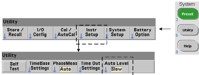
Auto-leveling is available for two input frequency ranges: 50 Hz to < 10 kHz and frequencies  $\geq 10$  kHz. The auto-level period is shorter for frequencies  $\geq 10$  kHz when an (auto-level) frequency range is set from the front panel or specified by the command:
