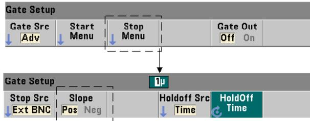
When using the external gate sources listed above, the polarity of the stop gate signal is set (changed) with the command:
