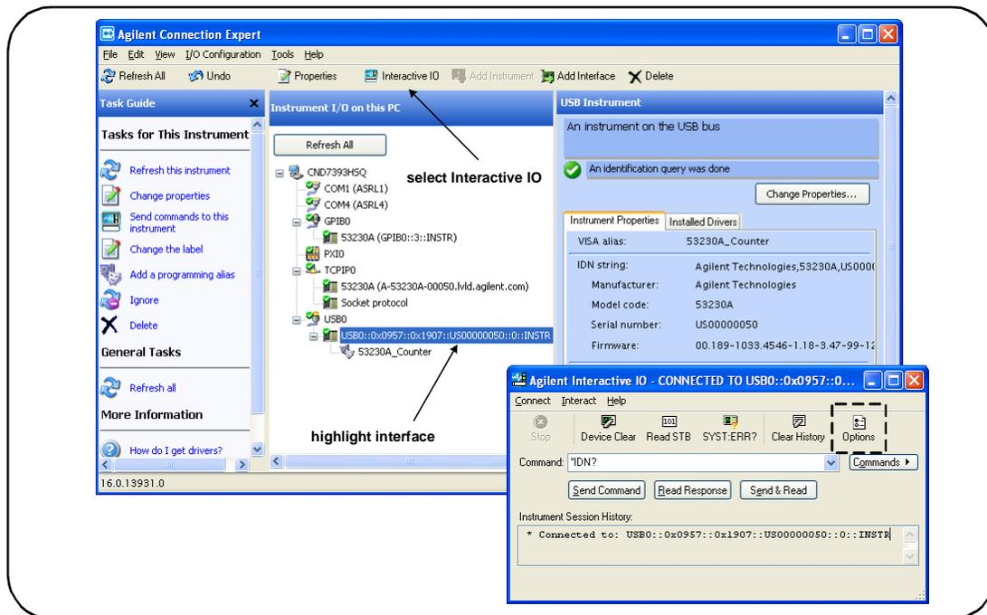
Figure 2-8. Starting Interactive IO for a Selected Interface.
