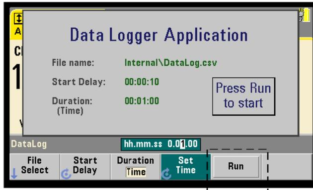
Pressing the Run softkey enables data logging. Data logging begins following any specified start delay when a valid path/file exists. A default path and file name of:
