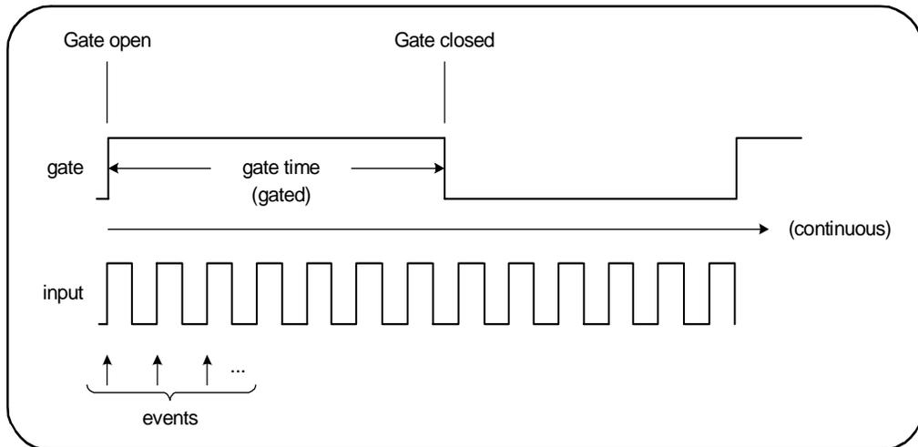
**Figure 3-12. Gated and Continuous Totalizing.**
