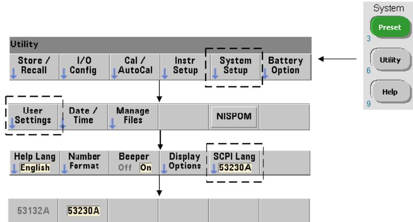
The 53220A/53230A's emulation mode enables the Agilent 53132A SCPI command set to be used with the counter.
