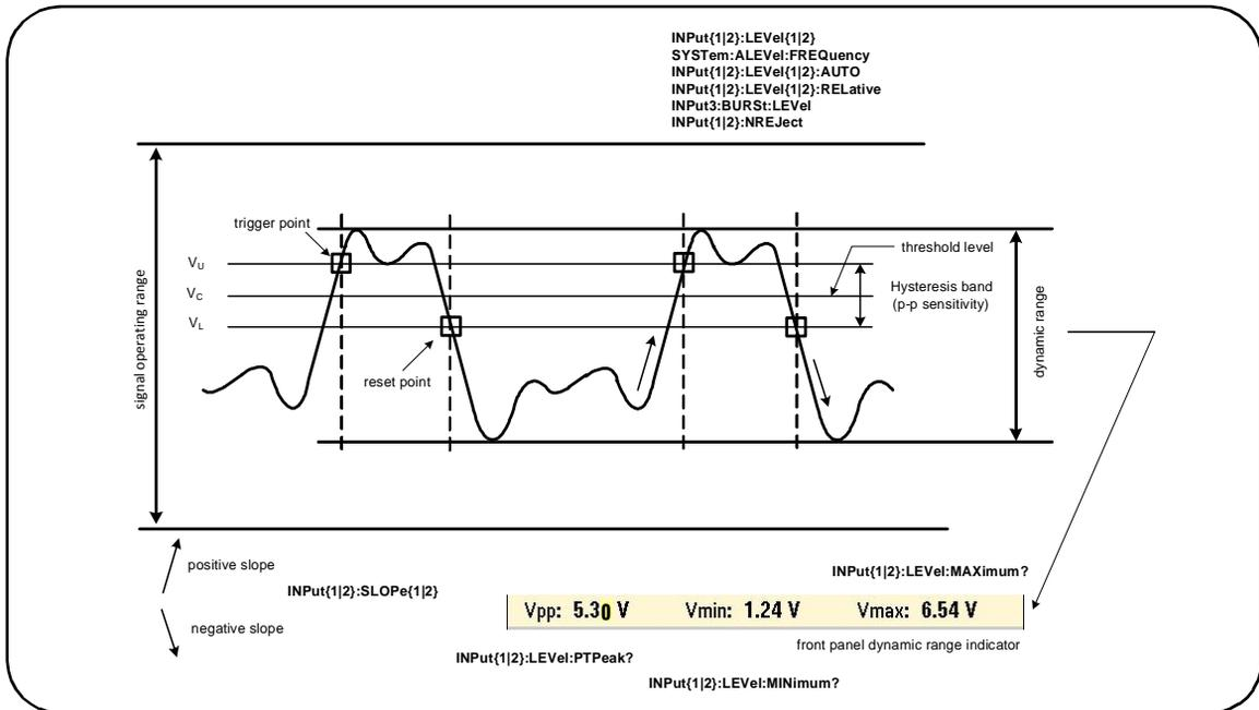
Figure 4-4. Input Signal Threshold Level and Sensitivity.
