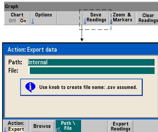
The readings represented by the trend chart can be saved to internal flash memory or to an external USB memory device as comma-separated values (CSV) in one measurement per line ASCII format.
