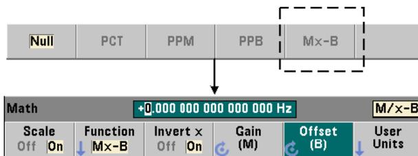
Scaling function results must be in the range of  $-1.0\text{E}+24$  to  $-1.0\text{E}-24$ ,  $0.0$ , or  $+1.0\text{E}-24$  to  $1.0\text{E}+24$ . Results outside these limits will be replaced with  $-9.9\text{E}+37$  (negative infinity),  $0$ , or  $+9.9\text{E}+37$  (positive infinity).
