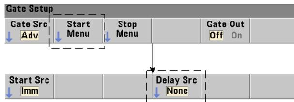
When using either an internal (immediate) or external signal to start (open) the gate, a delay from when the signal is received to when the gate is started (opened) can be specified. The delay source and its parameters are set with the commands:
