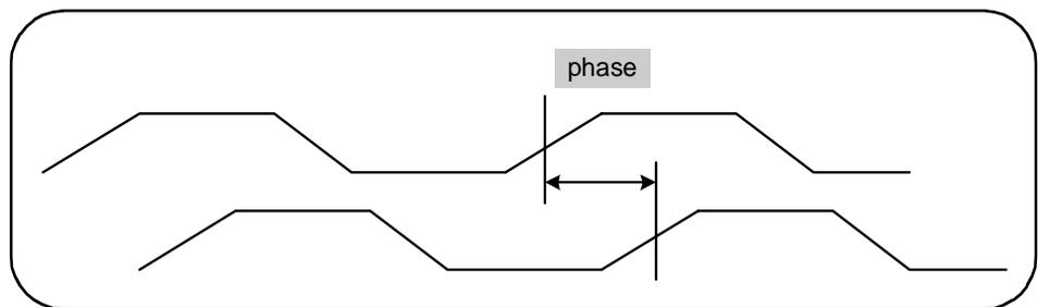
Figure 3-11. Phase Measurement Between Two Channels.
