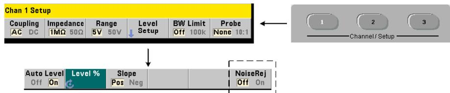
Threshold sensitivity (Figure 4-4) to the input signal is a function of the amount of noise rejection or hysteresis. Noise rejection (the hysteresis band) at the counter input is increased or decreased with the command:
