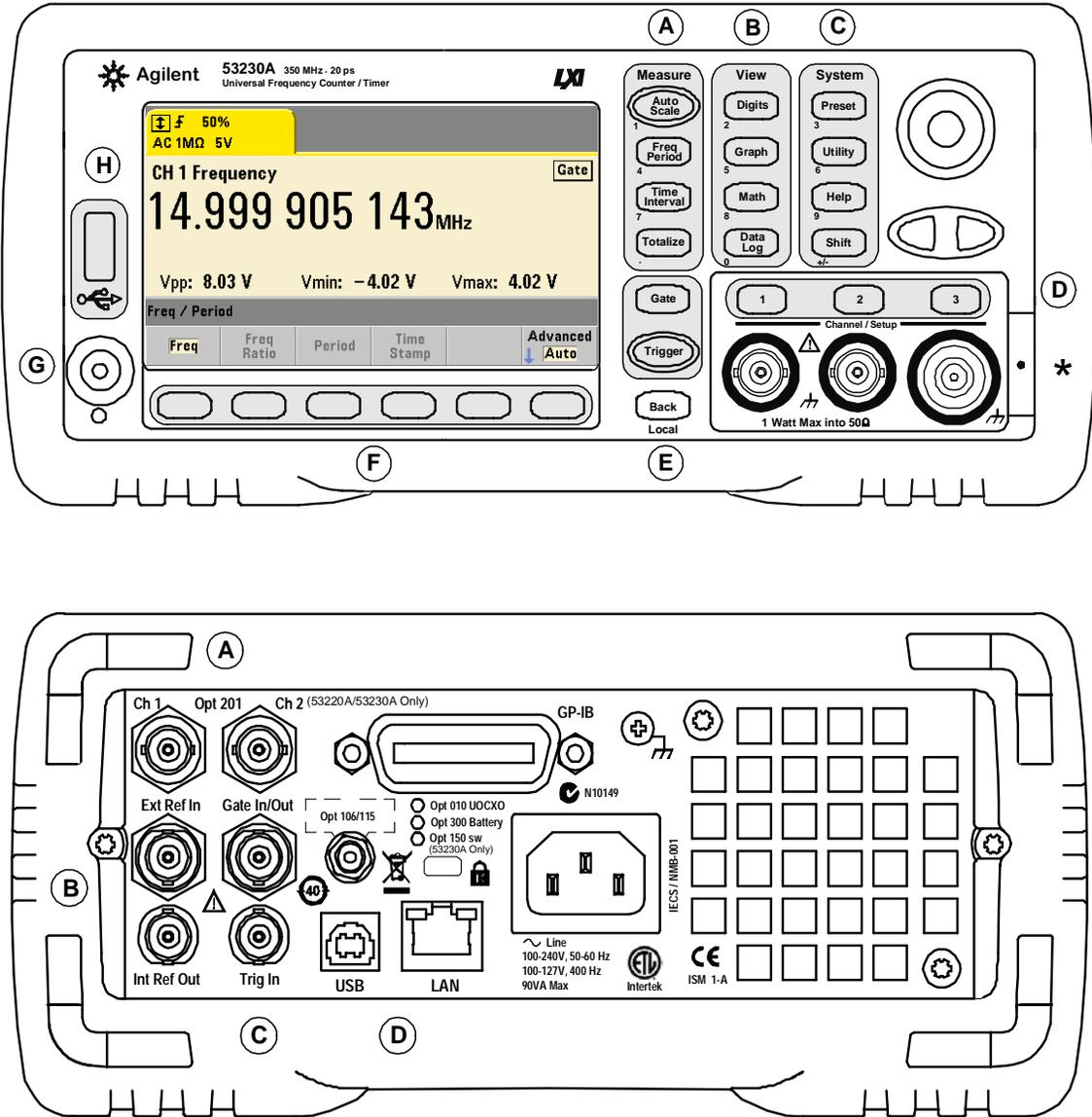
Figure 1-1. The 53220A/53230A Universal Frequency Counter/Timer.
