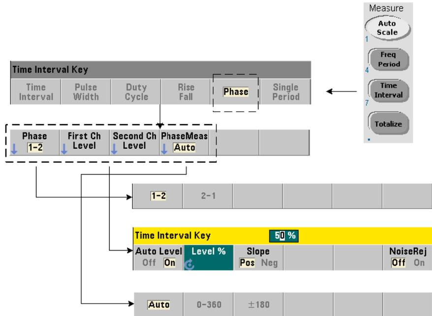
Phase measurements indicate the phase difference or shift between signals on counter channels 1 and 2 (Figure 3-11).
