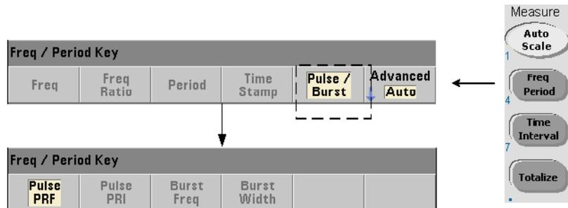
Microwave (burst) pulse measurements are available on channel 3 **Option 106** (6 GHz Microwave Input) or **Option 115** (15 GHz Microwave Input) with pulse measurement **Option 150**.
