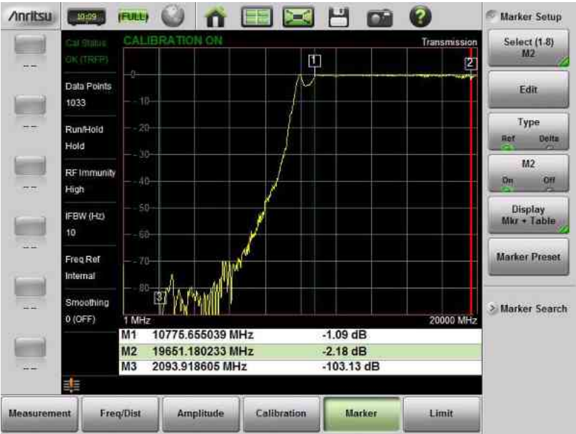
Figure 3-13. 2-Port Transmission Measurement Example, Waveguide
