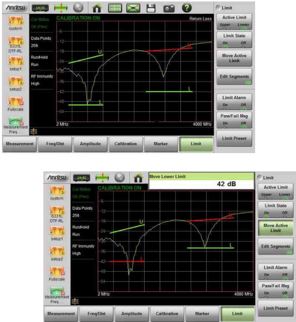
Figure 3-21. Moving Limit Line Segments
