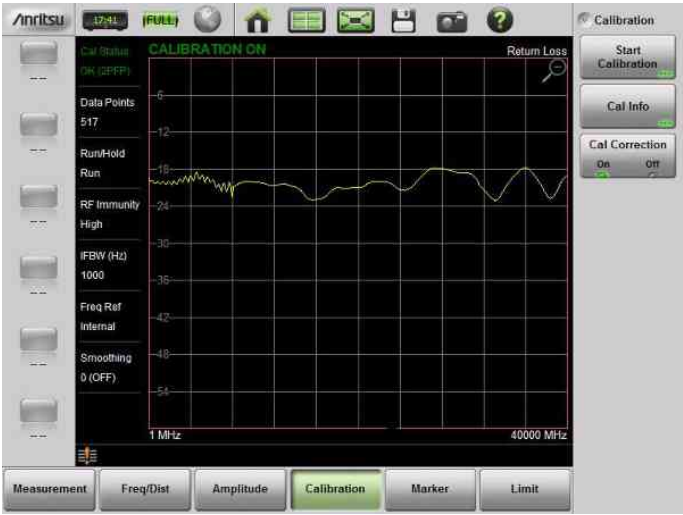
Figure 4-2. Return Loss Measurement after Calibration
