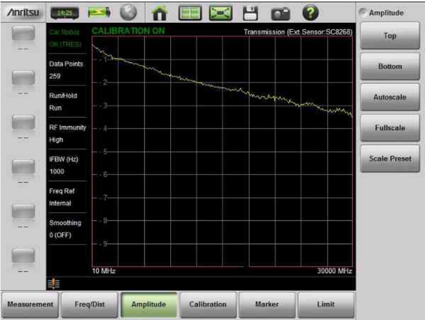
Figure 3-15. External Sensor Transmission Measurement Example
