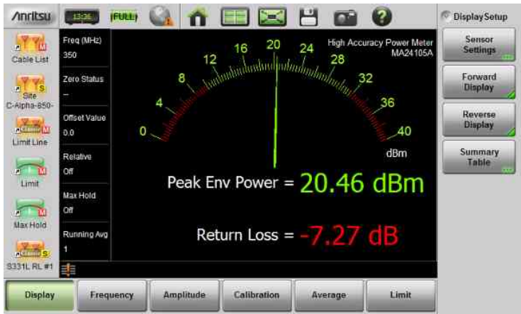
Figure 9-6. Power Meter View
