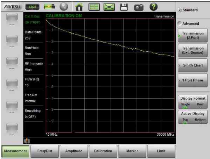
Figure 3-14. 2-Port Transmission Cable Loss Measurement Example
