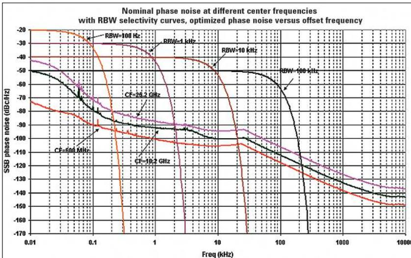
Figure 1. Nominal phase noise at different center frequencies
