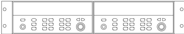
**To rack mount two instruments side-by-side, order lock-link kit 5061-9694 and flange kit 5063-9212. Be sure to use the support rails inside the rack cabinet.**
