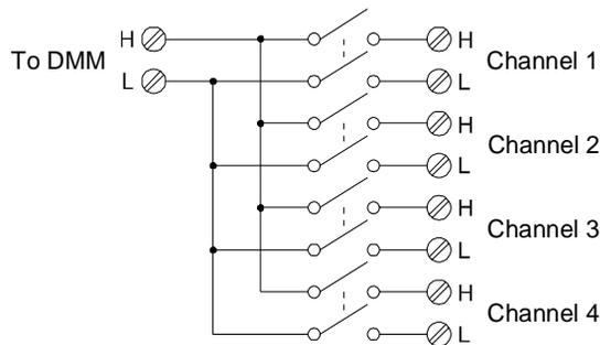
Note: If any channels are configured to be part of the scan list, you cannot close multiple channels; closing one channel will open the previously closed channel.
