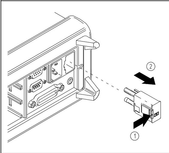
**2 Remove the line-voltage selector from the assembly.**
