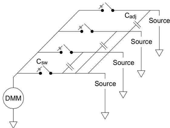
Capacitive noise coupling is a function of area and proximity. A simple method to reduce the noise coupling is to physically separate the switches and cables from each other. However, this may not be practical for all applications.
