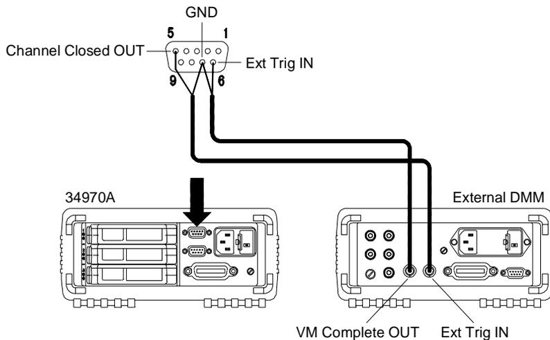
In this configuration, you must set up a *scan list* to include all desired multiplexer or digital channels. Channels which are not in the list are skipped during the scan. The instrument automatically scans the list of channels in ascending order from slot 100 through slot 300.
