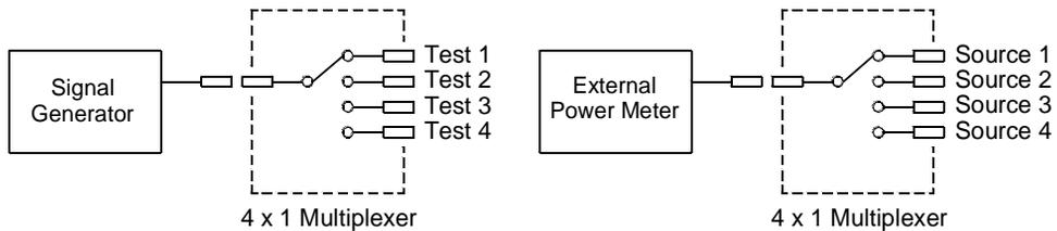
By using patch cables, you can expand RF multiplexers to provide additional test inputs or outputs. For example, you can combine two 4-to-1 multiplexers to create a 7-to-1 multiplexer as shown below.
