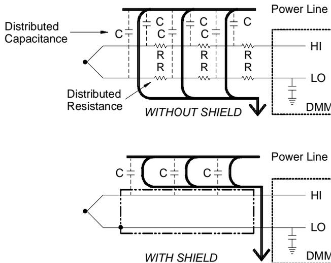
Common mode noise can dramatically affect the internal DMM. A typical thermocouple output is a few millivolts and a few millivolts of common mode noise can overload the input to the internal DMM.
