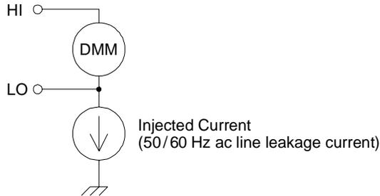
With *Connection A* (see below), the injected current flows from the earth connection provided by the circuit to the LO terminal of the internal DMM. This configuration adds no noise to the measurement. However, with *Connection B*, the injected current flows through the resistor  $R$  thus adding noise to the measurement. With *Connection B*, larger values of  $R$  will make the problem worse.
