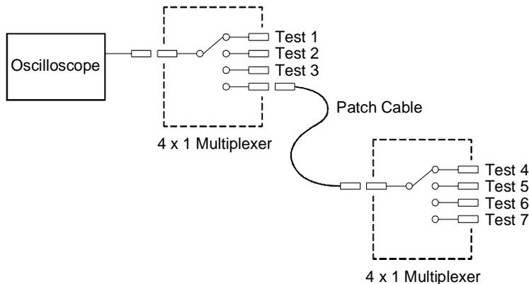
On the 34905A (50Ω) and 34906A (75Ω) RF multiplexers, you can close only one channel per bank at a time; closing one channel in a bank will open the previously closed channel. These modules respond *only* to the CLOSE command (OPEN does not apply). To open a channel, send the CLOSE command to another channel in the same bank.
