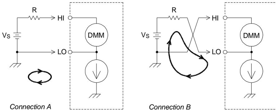
The measurement noise caused by injected current can be significantly reduced by setting the integration time of the internal DMM to 1 PLC or greater (see page 103 for a discussion of integration time).
