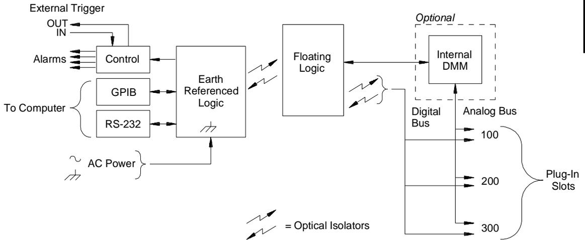
The earth-referenced and floating circuitry communicate with each other via an optically-isolated data link. The earth-referenced section communicates with the floating section to provide PC connectivity. The instrument is shipped with both an GPIB (IEEE-488) interface and an RS-232 interface. Only one interface can be enabled at a time.
