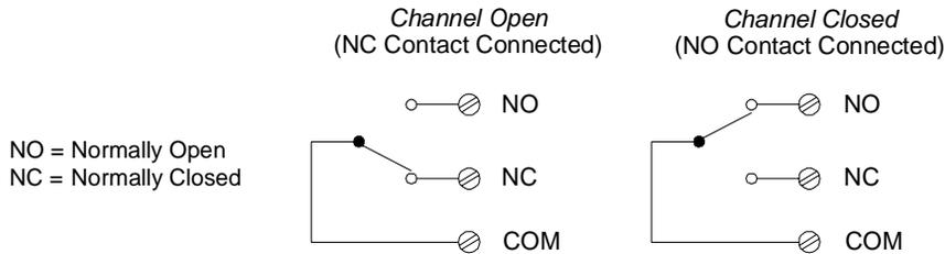
Each channel can switch up to 300V dc or ac rms. Each switch can also switch up to 1 A dc or ac rms up to 50 W maximum. For example, the maximum current that you can switch at 120 V is 0.45 A as shown below.
