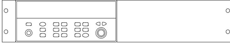
**To rack mount a single instrument, order adapter kit 5063-9240.**
