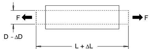
**Stress** Stress is a term used to compare the loading applied to a material with its ability to carry the load. Stress ( $\sigma$ ) in a material can not be measured directly; it must be computed from material properties and measurable quantities such as strain and force.
