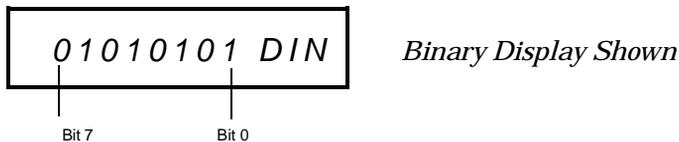
The bit pattern read from the port will be displayed until you press another key, turn the knob, or until the display times out.
