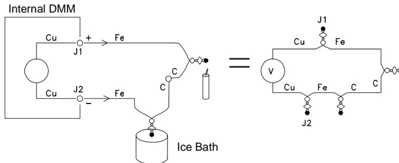
Two additional thermocouples have been created where the iron (Fe) lead connects to the internal DMM's copper (Cu) input terminals. Since these two junctions will generate opposing voltages, their effect will be to cancel each other. However, if the input terminals are not at the same temperature, an error will be created in the measurement.
