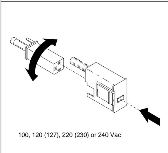
**4 Replace the fuse-holder assembly in the rear panel.**
