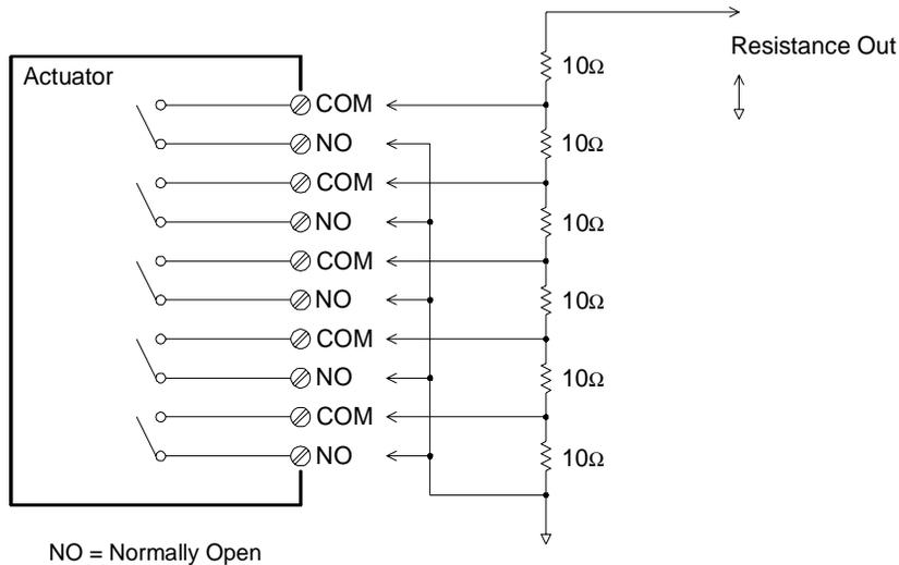
In the above diagram, the resistance is 60Ω when all of the actuator channels are open (not connected to COM). Note that when the actuator channels are open, as shown above, the normally-closed contacts (*not shown above*) are connected to COM. Values from 10Ω to 50Ω are selected by closing the appropriate channel(s) on the module.
