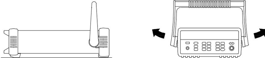
To remove the handle, rotate it to the vertical position and pull the ends outward.
