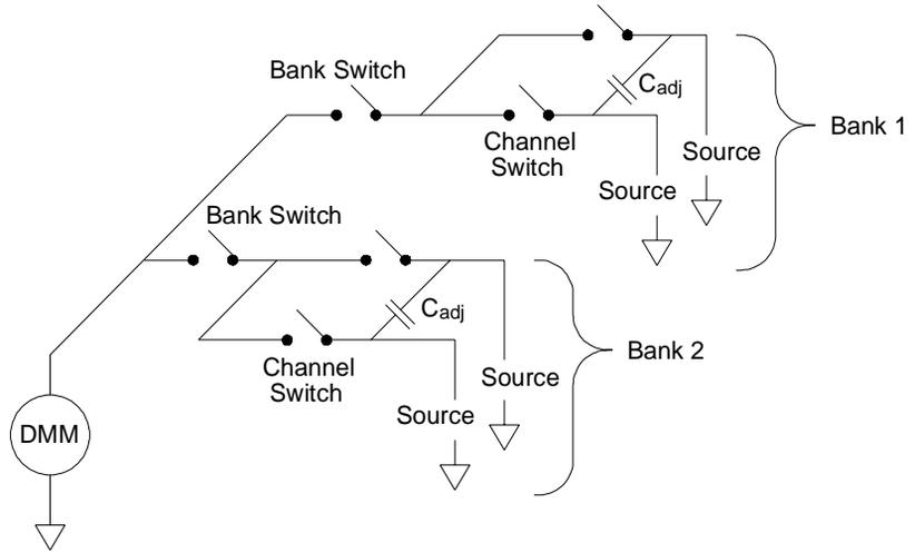
If you are not using all of the channels on the multiplexer, divide the input signals equally between Bank 1 and Bank 2. For example, if you are multiplexing eight channels using the 16-channel multiplexer, use four channels in the lower bank and four channels in the upper bank. For even better noise immunity, leave one unused, grounded channel between each input channel.
