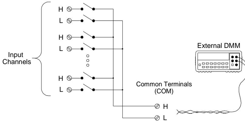
To control scanning with an external instrument, two control lines are provided. When the 34970A and the external instrument are properly configured, you can synchronize a scan sequence between the two.
