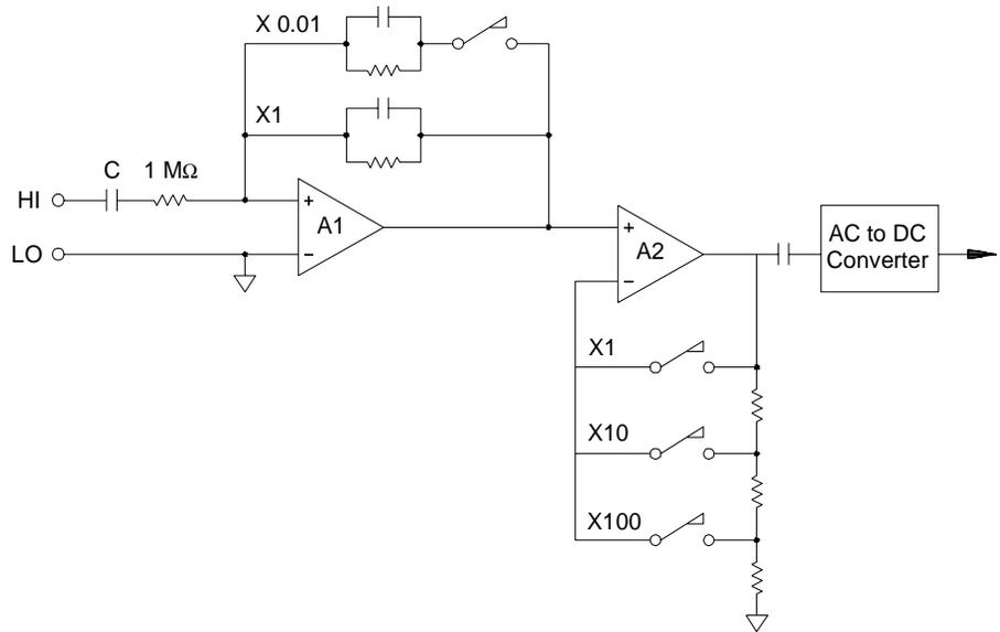
The first stage implements a high input impedance (1 MΩ) switchable compensated attenuator. The second stage provides variable-gain signal amplification to scale the input to the ac converter to the full-scale level. Any residual dc offset from the attenuator and amplifier stages is blocked by a capacitor.
