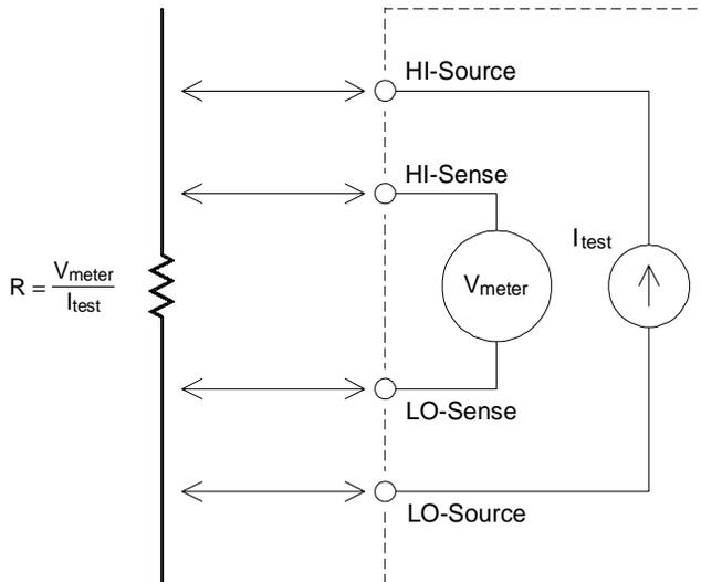
**Offset Compensation** Most connections in a system use materials that produce small dc voltages due to dissimilar metal-to-metal contact (thermocouple effect) or electrochemical batteries (*for a description of the thermocouple effect, see page 340*). These dc voltages also add errors to resistance measurements. The offset-compensated measurement is designed to allow resistance measurements in the presence of small dc voltages.
