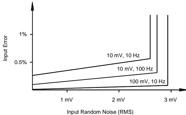
If the external noise pickup becomes large enough to exceed the hysteresis of the measuring circuitry, the frequency function may actually become unusable. External shielding and low-pass filtering may help.
