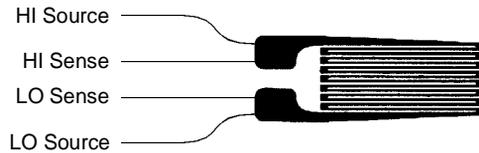
**Common Uses for Strain Gages** Strain gages are used to sense many types of physical parameters. Strain gages are primarily a force-sensing device. Force is measured indirectly by measuring the deformation of a test body to a known applied force thus producing a resistance change proportional to the applied force. Many other physical quantities can be measured through force measurements. Common applications of strain gages include weight, pressure, flow, and level measurements.
