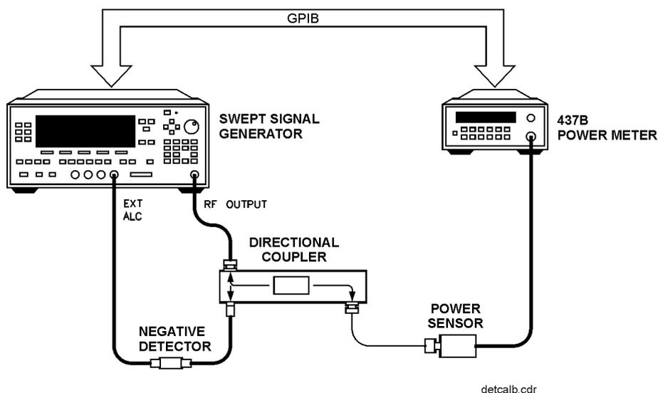
Figure 1-22. Automatically Characterizing and Compensating for a Detector
