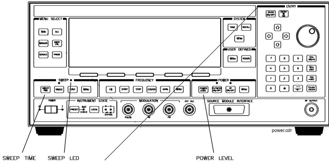
**Figure 1-6. Power Level and Sweep Time Operation**
