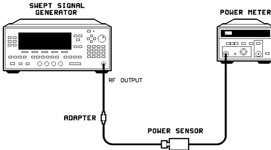
Figure 1-10. Power Sweep and Power Slope Operation
