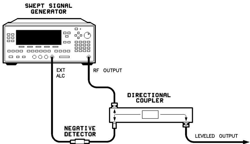
Figure 1-11. ALC Circuit Externally Levelled
