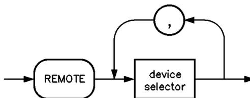
where the device selector is the address of the instrument appended to the GPIB port number. Typically, the GPIB port number is 7, and the default address for the swept signal generator is 19, so the device selector is 719. Some BASIC examples:
