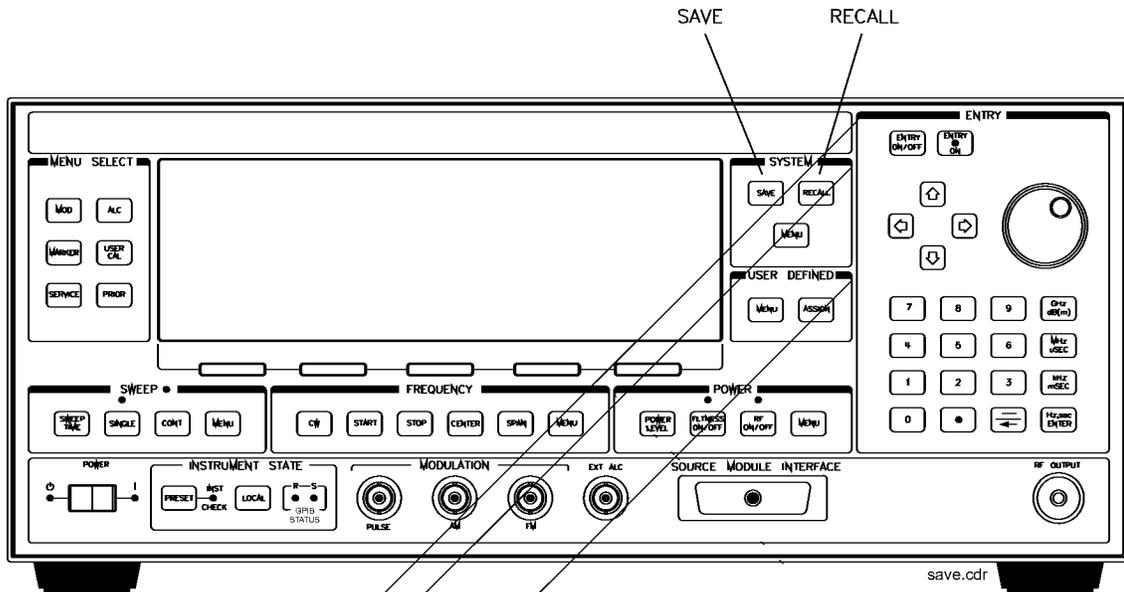
Figure 1-9. Saving and Recalling an Instrument State
