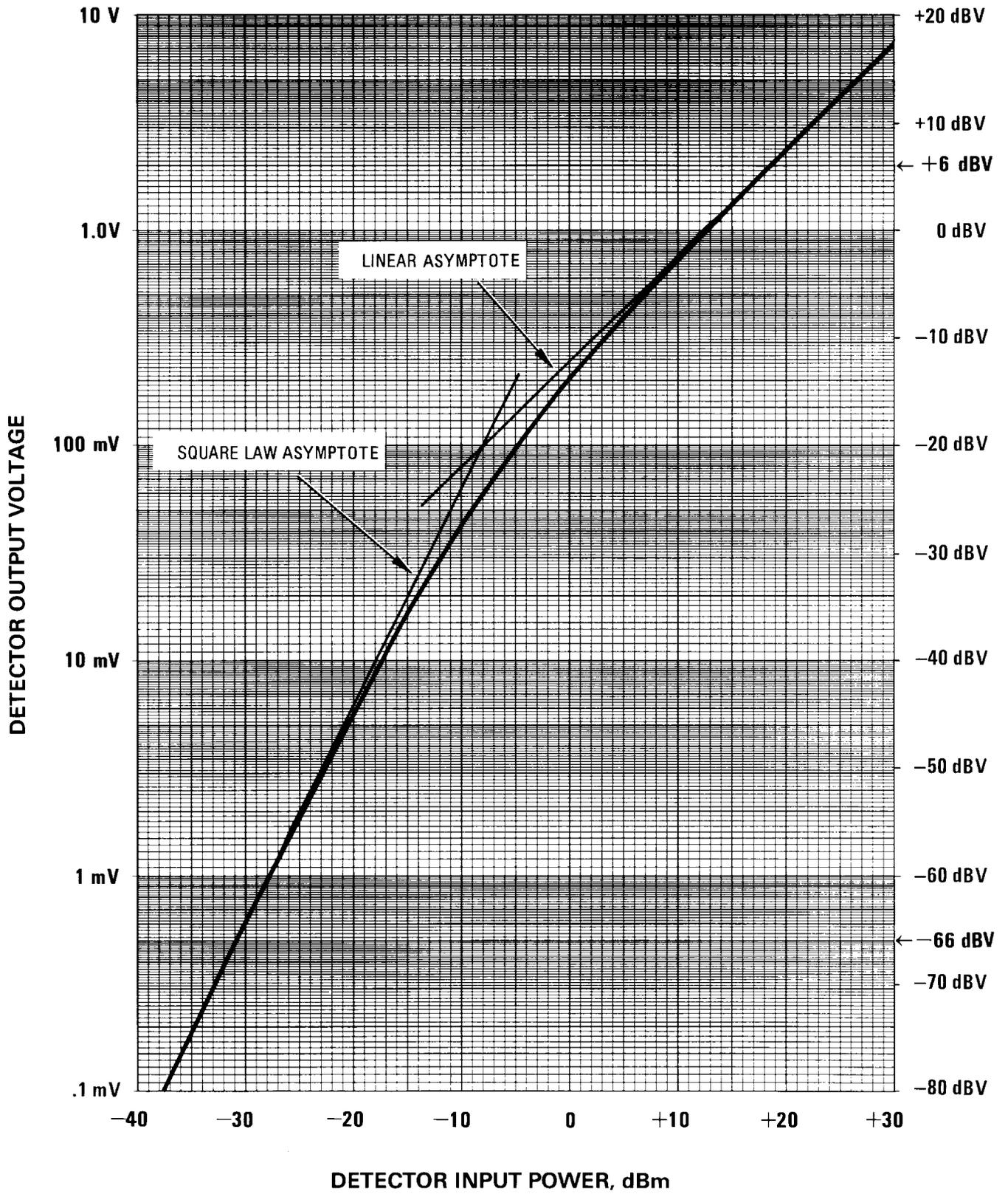
Figure 1-12. Typical Diode Detector Response at 25°C
