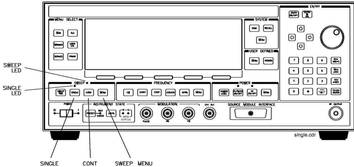
**Figure 1-7. Continuous, Single, and Manual Sweep Operation**
