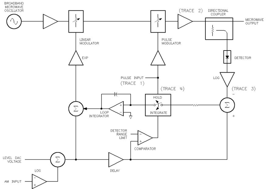
Figure M-4. ALC Block Diagram
