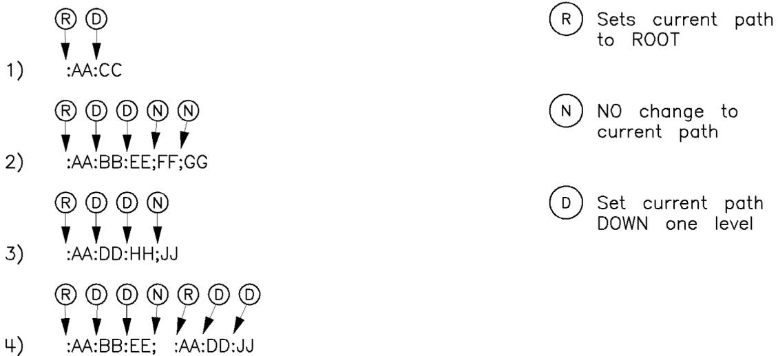
**Figure 1-26. Proper Use of the Colon and Semicolon**
