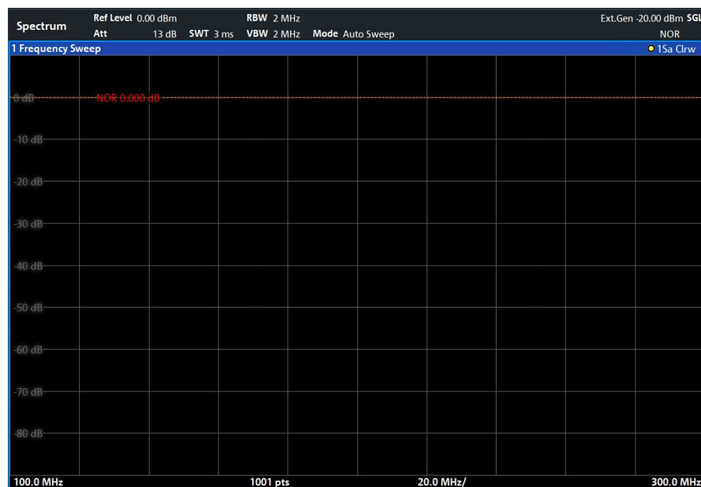
Figure 7-9: Normalized measurement results after calibration
