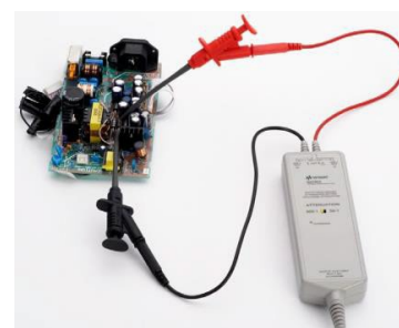
N2790A measuring a power supply signal
