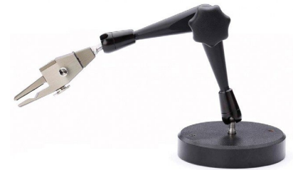
N2787A 3D probe positioner
