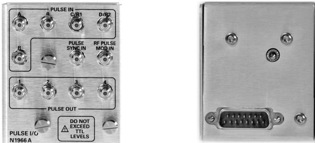
Figure 5. Pulse I/O adapter (N1966A) simplifies connections
