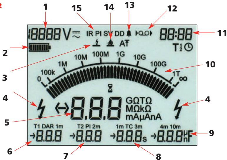
1. **Voltage at terminals** — Displays amount of voltage present at the terminal.
