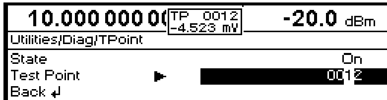
Fig. 4-41 Utilities – Diag – TPoint menu
