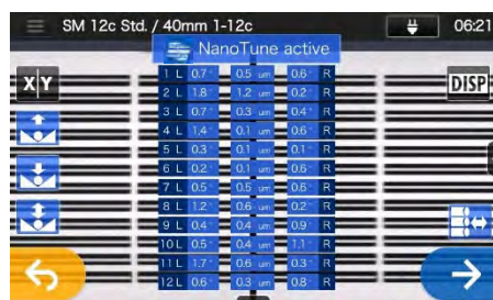
2: Inspection of fiber end face. The NanoTune™ is activated when the end face is poor.
