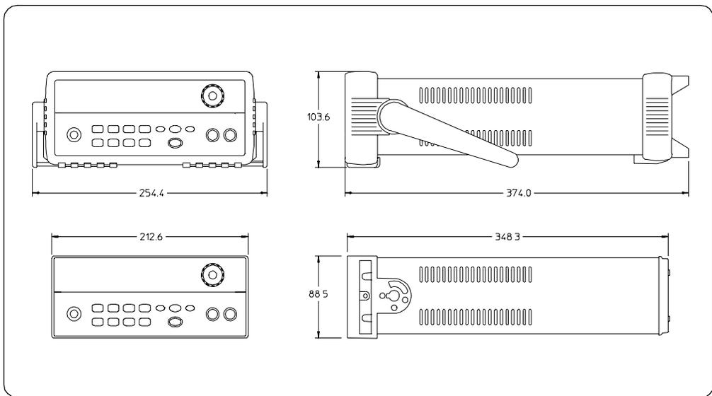
**Figure 8-1. Dimensions of Agilent E3640A/41A/42A/43A/44A/45A Power Supply**
