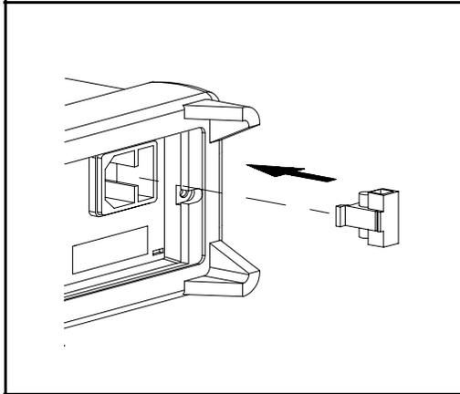
**Verify that the correct line voltage is selected and the power-line fuse is good.**
