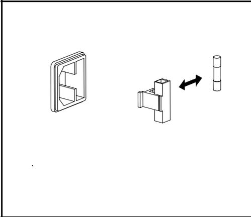
**4 Replace the fuse-holder assembly in rear panel.**
