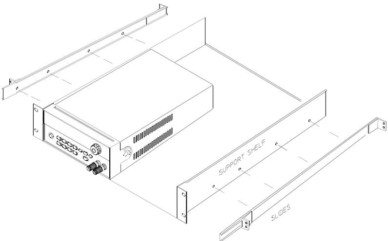
To install two instruments in a sliding support shelf, order support shelf 5063-9255, and slide kit 1494-0015.
