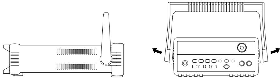
To remove the handle, rotate it to the vertical position and pull the ends outward.
