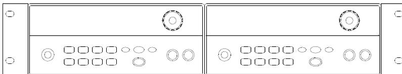
To rack mount two instruments side-by-side, order lock-link kit 5061-9694 and flange kit 5063-9212. Be sure to use the support rails inside the rack cabinet.
