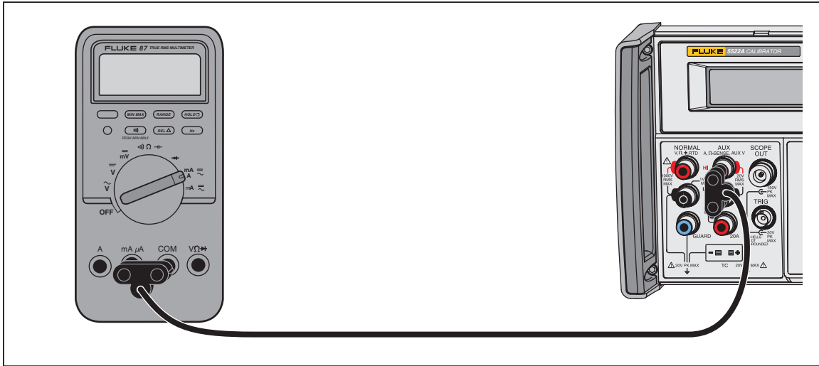
Figure 4-8. UUT Connection: DC Current/AC Current
