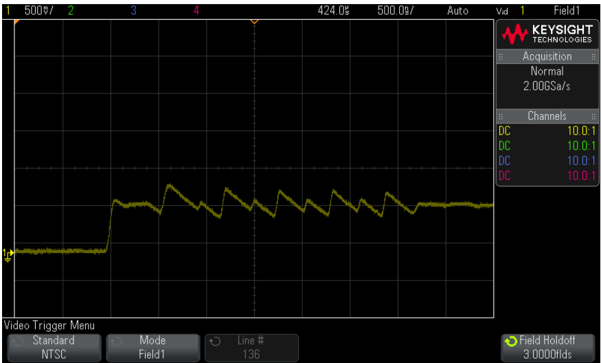
Figure 32 Using Field Holdoff to Synchronize to Color Field 1 or 3 (Field 1 mode)
