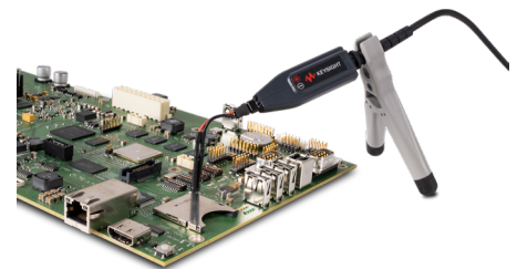
DP001xA Series probe using socketed Y-lead
