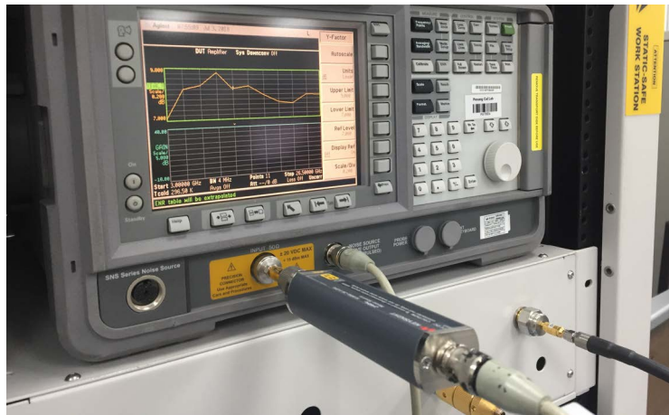
Figure 4-4 Operator's check test setup 2b
