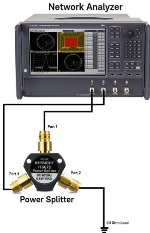
Figure 4-3 Output tracking test setup (Port 2 Terminated)
