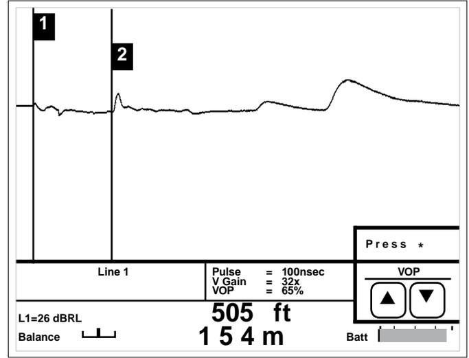
After the first major reflection, the second event could be a more severe fault. It appears smaller due to absorption of signal at the first fault. Always shoot the cable from both ends to eliminate this problem.
