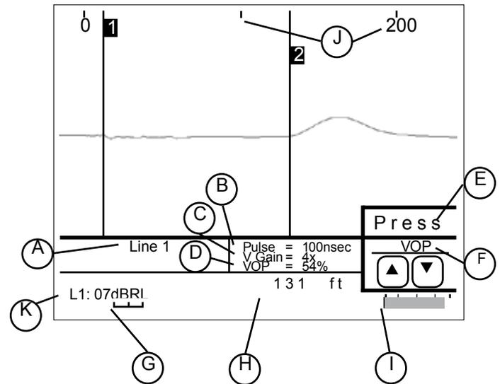
F. SELECTED MENU ITEM. Displays the currently active menu selection, which is controlled by the icon keys. The on-screen icons graphically represent how the keys affect the control.
