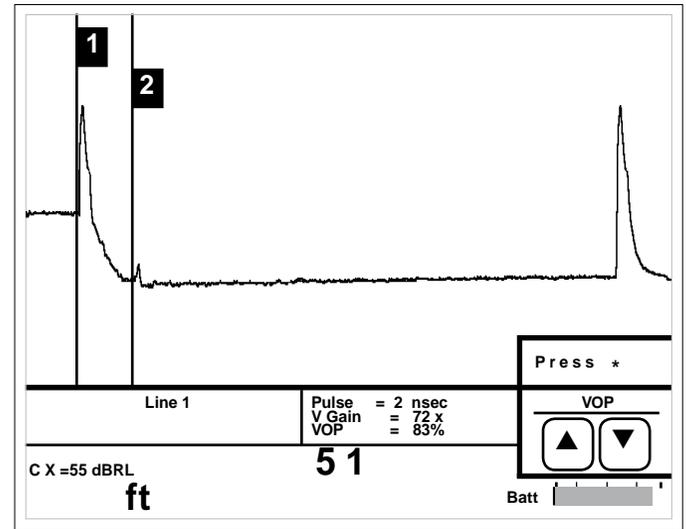
Two sections of cable with a splice shown at the 2nd cursor. The amount of reflection caused by the splice is directly proportional to the quality of the splice. A good splice = small reflection; a bad splice = large reflection.
