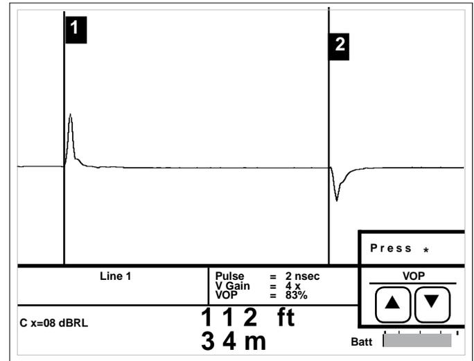
A reflection with the opposite polarity indicates a fault with short (low impedance) tendencies. The reflection shown at the 2nd cursor is a dead short.
