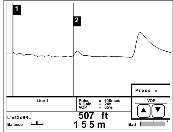
The middle reflection at the 2nd cursor is a ONE SIDE PARTIAL OPEN followed by a COMPLETE OPEN (end of the cable). The more severe the fault, the larger the reflection will be.
