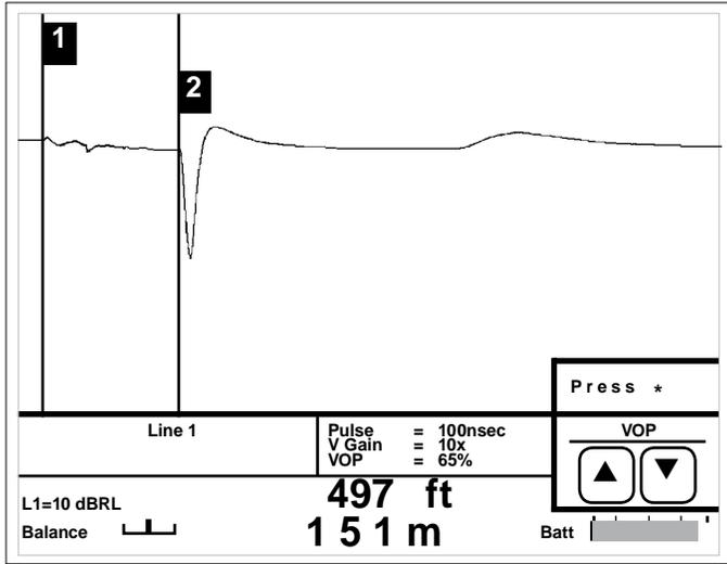
A telephone BUILD-OUT CAPACITOR causes a low impedance DOWNWARD reflection (similar to a SHORT) followed by a smaller positive reflection.
