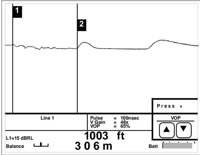
A 10 Ohm series resistance fault at the 2nd cursor (1003 feet) followed by a complete open at 2000 feet.
