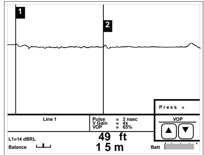
A joint or splice at the 2nd cursor. The visibility of a splice will depend on the type and quality of the splice, and the distance away.
