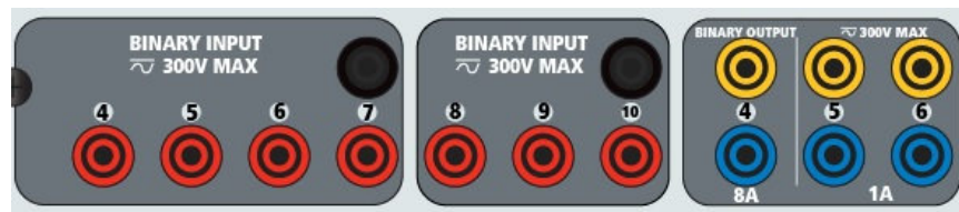
Figure 400 Binary Inputs 4 to 10 and Binary Outputs 4 to 6
