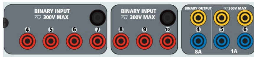
Figure 369 Binary Inputs 4 to 10 and Binary Outputs 4 to 6
