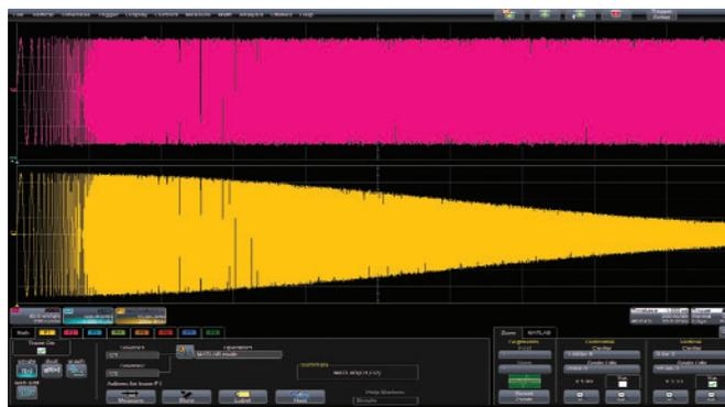
*XDEV allows MATLAB® script to apply a customized filter and return the waveform to the scope display. Continue further analysis with the advanced toolbox in the oscilloscope.*
