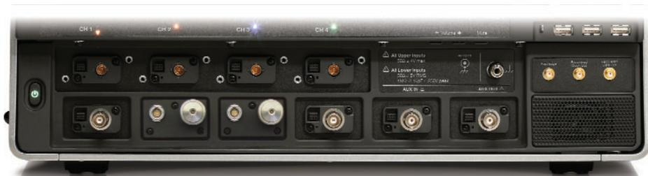
*The 8 inputs can essentially be multiplexed into four channels to minimize probe reconnections or to simplify automated testing.*
