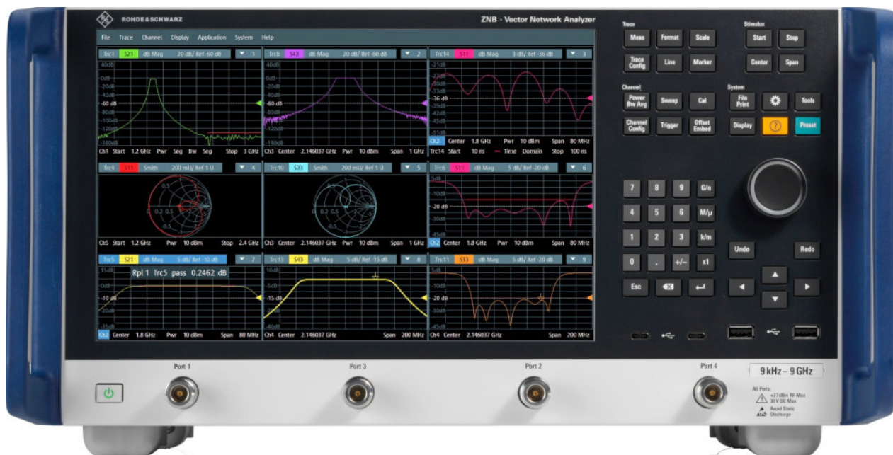
Figure 3-1: R&S ZNB3004 with four ports
