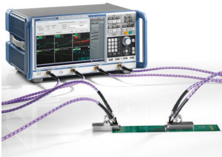
Figure 4-14: Test setup for fixture deembedding
