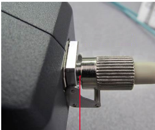
Correct way of connecting - Keying features are proper aligned
