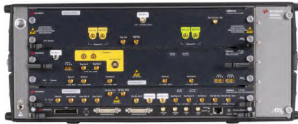
M8042A (1-channel), M8009A, M8053A in single chassis
