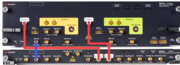
Figure 16 Two-channel system using one M8042A pattern generator (two channels) and one M8009A clock module
