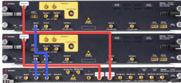
Figure 17 Two-channel system using two M8042A pattern generator (one channel) and one M8009A clock module
