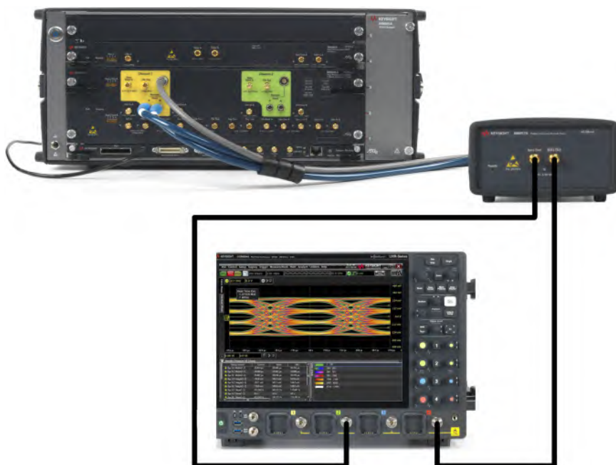
Connection among M8045A, M8057A/B and UXR-series oscilloscope
