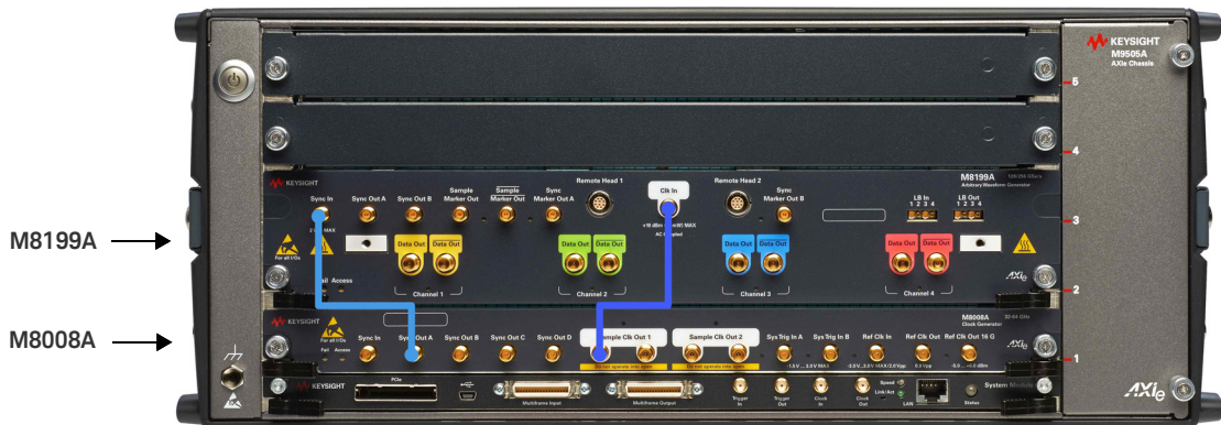
Figure 58 Connecting M8008A clock generator to M8199A AWG module
