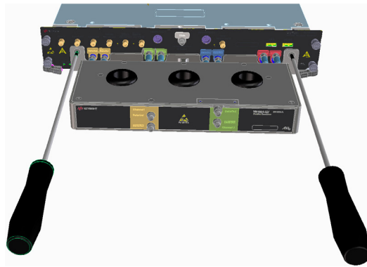
Figure 56 Fixing M8199A-ILV to M8199A using screws
