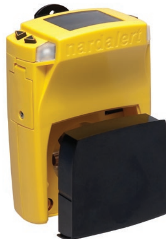
Nardalert S3 Mainframe shown with interchangeable sensor.
