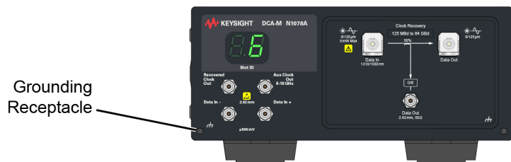
Figure 17. Grounding Receptacle on a DCA-M Instrument
