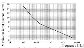
Fig. 2 Derating according to frequency
