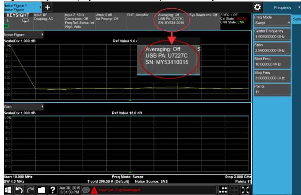
Signal Analyzer Display after USB Preamplifier is Ready For Use
