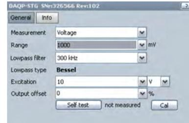
In the quarter bridge 4-wire mode the DAQP-STG internally adjusts its excitation so that on the gage the resistor terminates exactly on the half of the excitation voltage. All wire resistances are compensated.
