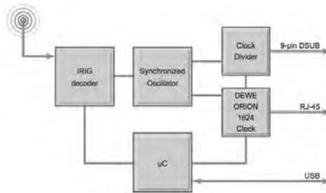
The IRIG-DECODER engine generates one pulse per second (PPS) which is used to synchronize a 40 MHz oscillator with software PLL (phase locked loop). The result is an ultra stable 40 MHz clock source which is completely free of drift over time.
