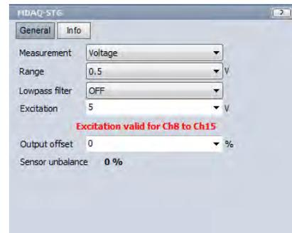
⇒ **CAUTION: If the excitation is not used for sensor supply it has to be deactivated by setting it to 0V.**
