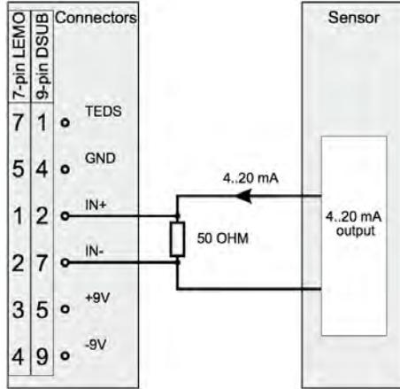
Current loop-powered measurement with external shunt
