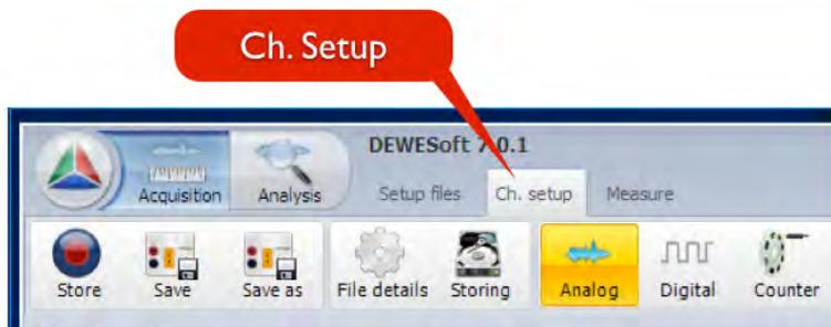
When you do this, you will be on the **ANALOG** setup screen first. This is where you set up the analog inputs of your system. You might have other setup screens for **DIGITAL**, **COUNTER**, **CAN**, **VIDEO** and more inputs... but let's focus on the analog inputs in this QuickStart. Notice that the Analog screen is highlighted in yellow when selected.
