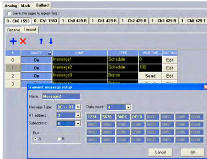
Every message has the Edit button which opens Transmit message setup form where all message properties and data can be set.
