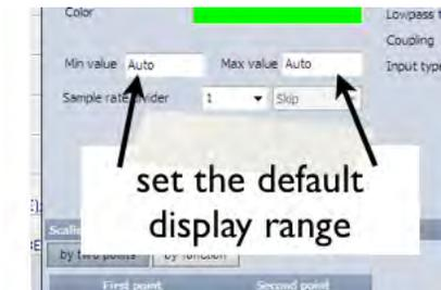
So in our example, we want the temperature channel's default range to be  $-100^{\circ}\text{F}$  to  $\pm 400^{\circ}\text{F}$ , therefore we would enter that like this:
