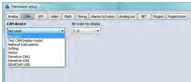
Use the selector to choose the CAN device that is installed within your system. Here is a basic description of what each entry refers to:
