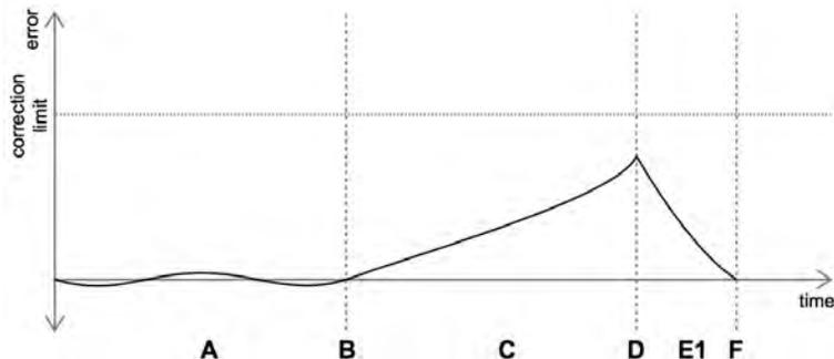
A) This state shows the normal operation. The internal clock is synchronized to the GPS once per second.
