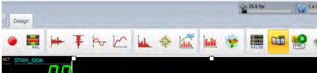
The video widget is shown highlighted in yellow, above. After you click it to add a video window, you can select any USED video streams from the channel list to put them onto your screen. The video widget can be scaled and moved freely into an attractive arrangement on your display:
