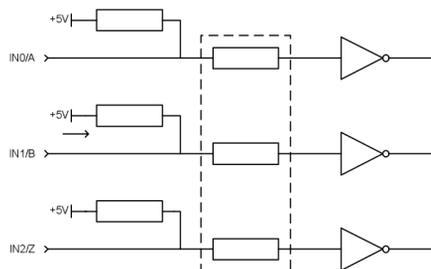
1) Pull-up resistors 2) Over-voltage protection 3) Buffers
