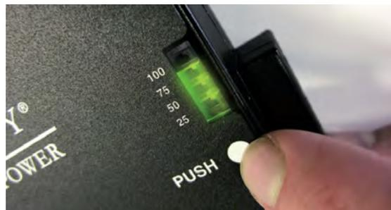
Press the white dot on the battery and the charge percentage indicator will show the approximate remaining charge, in 25% steps.
