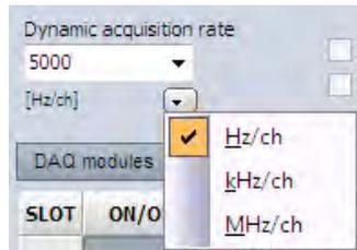
To select a rate, either choose one from the list that drops down from the little triangle, or simply type one into the field and press ENTER on the keyboard. If DEWESoft cannot do this range, it will correct it and show you what it can do:
