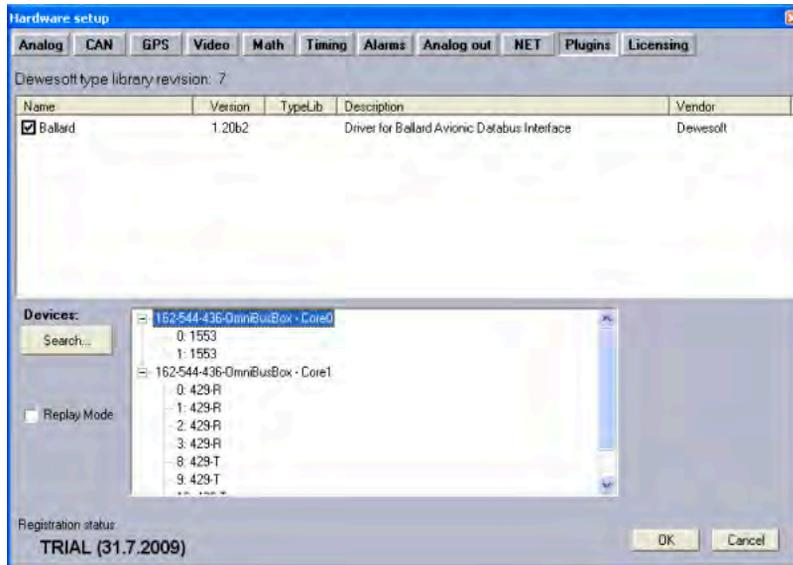
When this is done, the Ballard plugin will appear in Hardware setup plugin list.
