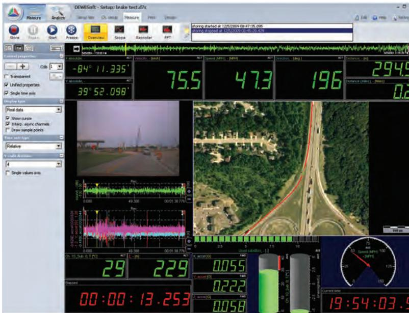
☺ **Note:** video streams also create a channel which contains the frame count. You can display this count in a digital meter as a convenience.
