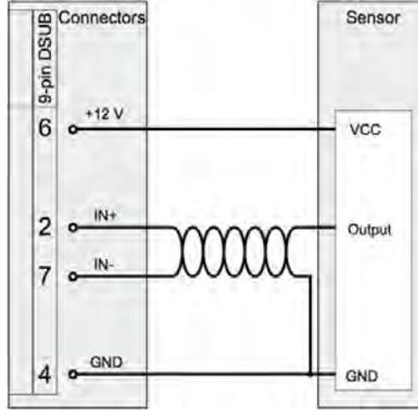
Loop-powered sensor, ext. shunt
