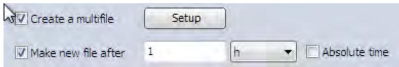
As before, DEWESoft can switch files automatically based on time (absolute or relative), file size, or trigger count. If you want one triggered event per data file, this is the way to do it, for example. Set it to triggers and set the quantity to 1.
