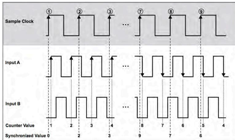
For X2 encoding the rising edges and the falling edges of Input A are used to increment or decrement. The counter increments if Input A leads Input B and decrements if Input B leads Input A.
