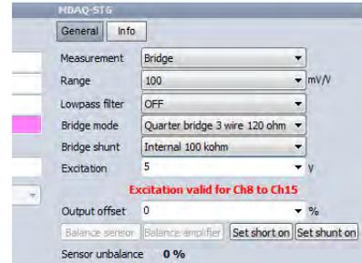
⇒ **Sense leads (SUB-D: pin 3 and 6 must be connected!**
