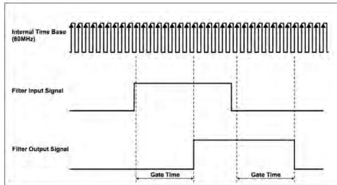
Below, input signal with chatter, before and after filtering:
