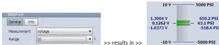
Now the measurement range of 10V yields a scaled measurement range of  $\pm 5000$  PSI, which is what you were looking for. In this way you can see the relationship between the ACTUAL hardware measuring range and the SCALED measuring range.
