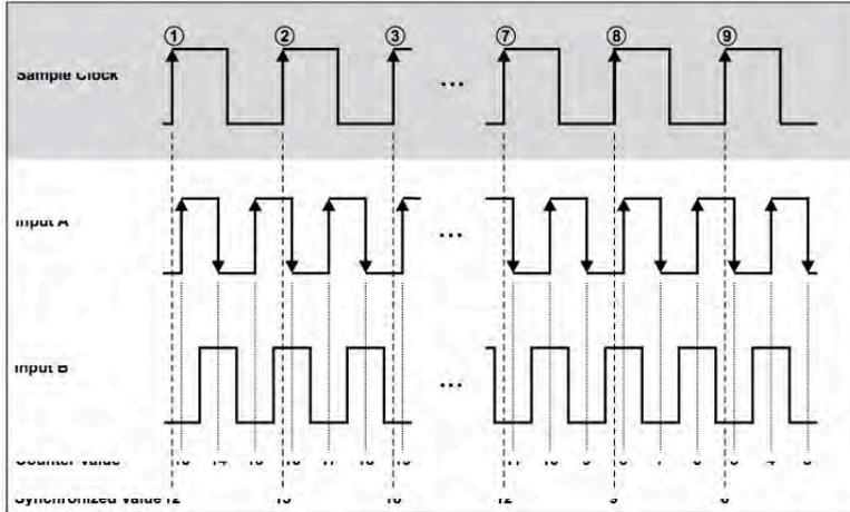
Similarly, the counter increments or decrements on each edge of Input A and Input B for X4 decoding. The condition for increment and decrement is the same as for X1 and X2.
