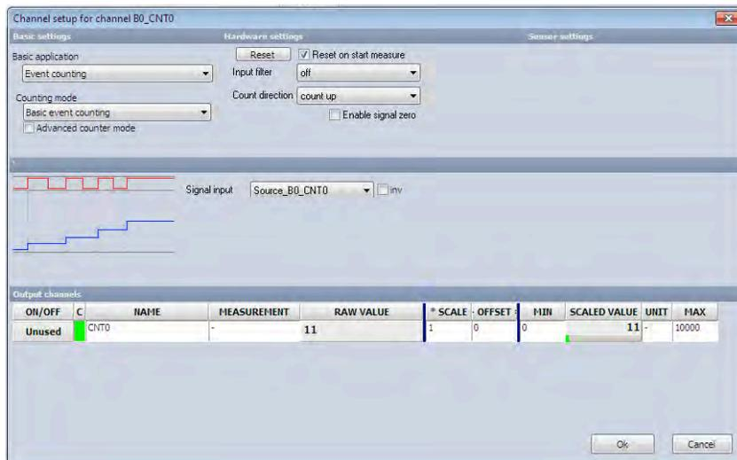
☺ If counting the falling edges is necessary, the input signal can be inverted.
