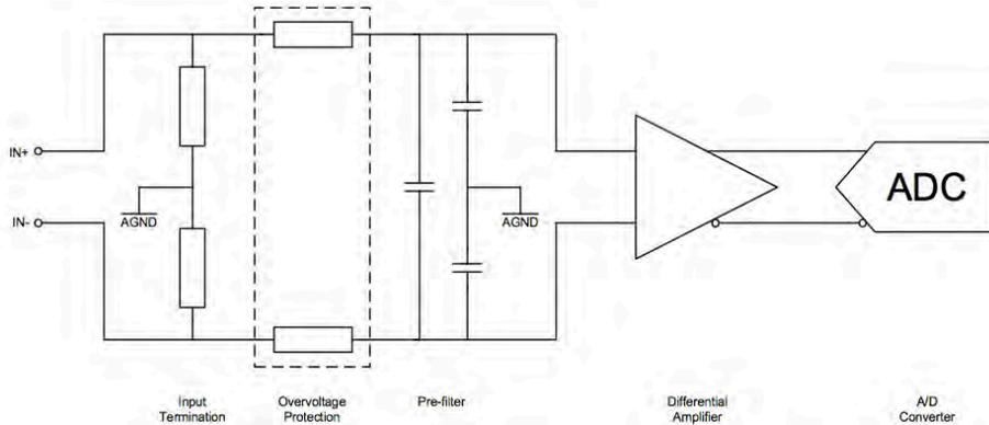
The high input impedance ( $10M\Omega$  ground referenced) has no distortion influence on the measured signal.
