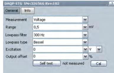
⇒ **CAUTION: If the excitation is not used for sensor supply it has to be deactivated by setting it to 0 V. This will internally connect the IN- to the GNDisolated to improve the common mode rejection.**
