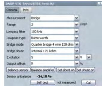
In the quarter bridge 4-wire mode the DAQP-STG internally adjusts its excitation so that on the gage the resistor terminates exactly on the half of the excitation voltage. All wire resistances are compensated.
