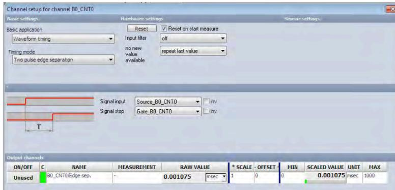
☺ If the input signals are inverted, the falling edges will be used for counting.
