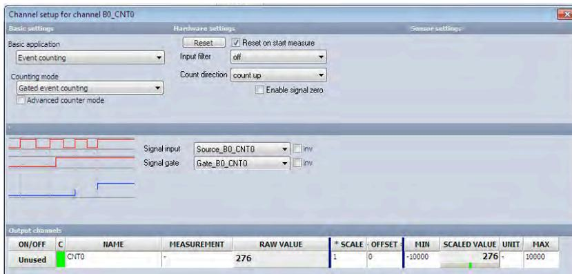
☺ If counting the falling edges is necessary, the input signal can be inverted.
