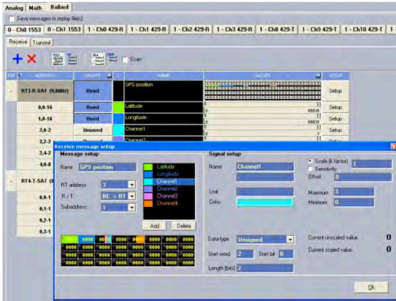
In the table you can see all messages, channels and live data. Messages are always ordered by their addresses. Some properties like color and name can be change directly on the table and for others you must open SETUP. In the SETUP dialog you can add channels and manage their properties.
