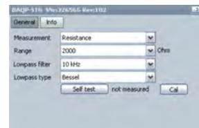
For resistance and RTD mode, 4-wire connection is recommended (2-wire connection will not compensate wire resistance).
