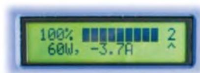
The battery status LCD keeps you informed of how many batteries are installed (2 above), the charge level (100% above), and whether the system is charging or discharging.
