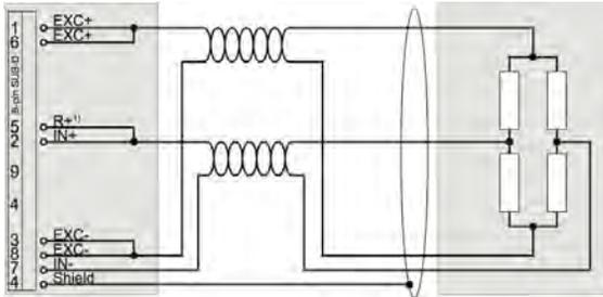
☺ Sense leads (SUB-D: pin 3 and 6) could be connected to be compatible to other modules.
