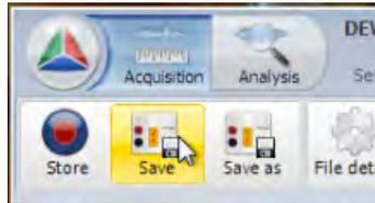
Everything that you can set up in DEWESoft is saved to a setup file that you can name freely (according to Windows file naming restrictions of course). It is ALWAYS a good idea to save your setup before moving on from here.
