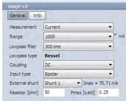
When you do this, the software changes the unit of measure from V to mA, and also presents you with the ability to select Shunt 1, Shunt 2 (Shunt 2 applies to Shunt 3, Shunt 4, and Shunt 5, which are the same electrically, but which only have different I/O connector configurations), as well as a variety of Dewetron specialized shunts for automotive applications:
