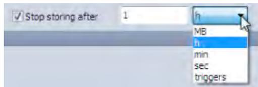
With Stop storing after checked, you can set DEWESoft to stop storing automatically based on time (hours, minutes, or seconds), or file size (in MB), or number of triggers within the file.
