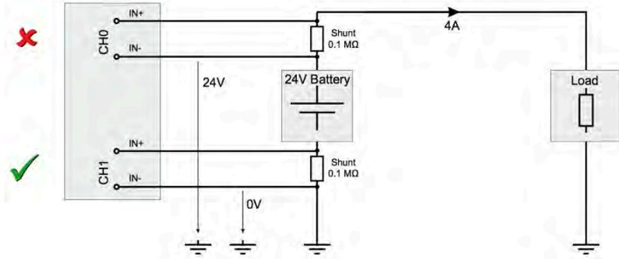
The optimum input range in that case is 500 mV. That will work fine for CH1 in the picture, but not for the CH0. This channel will exceed the maximum common mode voltage and go into overflow.
