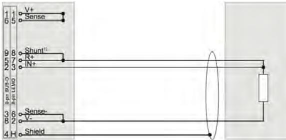
⇒ Sense leads (SUB-D: pin 3 and 6; LEMO: pin 5 and 6) **MUST** be connected!
