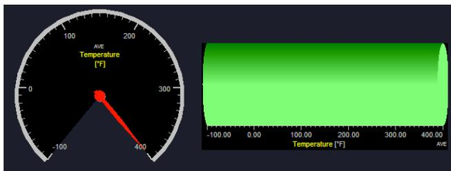
Above, the same temperature channel shown in several different kinds of graphs and meters, they all have the default  $-100^{\circ}\text{F}$  to  $+400^{\circ}\text{F}$  display scale, because you have preset the display scale back on the setup screen for that channel.
