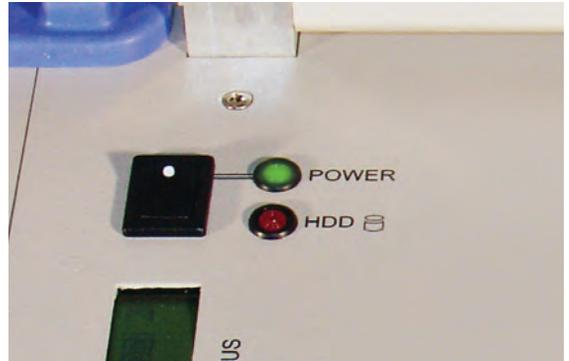
The DEWE-321x power switch is a momentary type, located on the front panel near the LED battery status display. To its right are LEDs for system power (green) and HDD activity (red).
