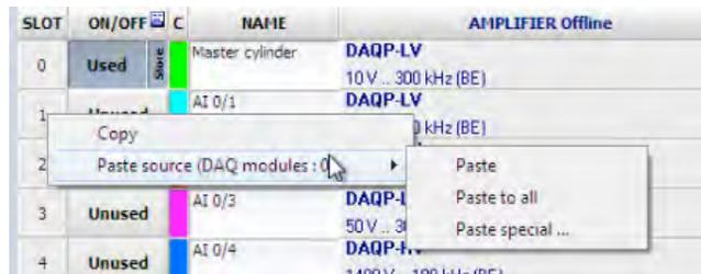
Now you get some very nice choices, which make the copy/paste process very flexible. Here is what each of the three sub choices under Paste source (<module type> : <channel>) means:
