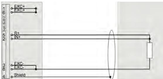
☺ Sense leads (SUB-D: pin 3 and 6) could be connected to be compatible to other DEWE-BRIDGE amplifier.
