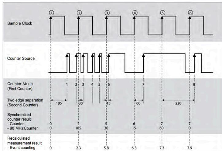
With these both measurement results not only the frequency can be calculated in a precise way. Also the event counter result can be show in fractions because the exact time when the event occurs at the input is known. The event counting result is recalculated with interpolation to the exact sample point like shown in the diagram above.
