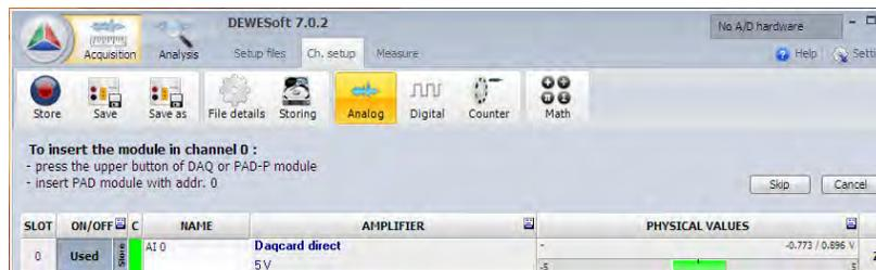
Follow the instruction to press the TOP black button on the module in the first slot, which is always SLOT 0 in the case of doing a FILL RACK, since you are starting at 0 and going all the way up, filling all modules.
