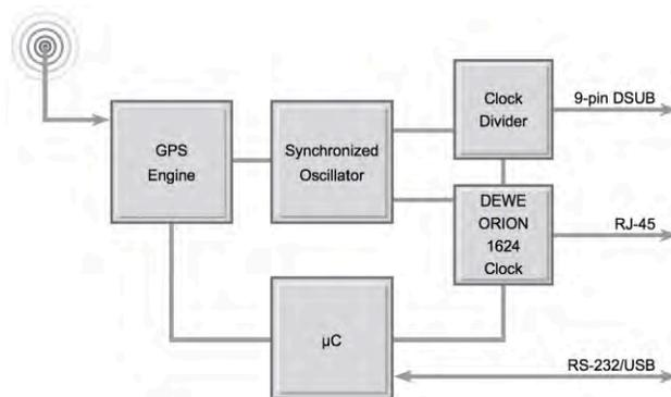
The base of any GPS receiver is precise time measurement. In addition to the position information a precise PPS (pulse per second) is generated by the GPS engine. This pulse is used to synchronize a 40 MHz oscillator with software PLL (phase locked loop). The result is an ultra stable 40 MHz clock source which is completely free of drift over time.
