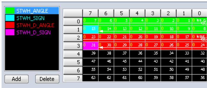
Or, if this message contains multiple channels, repeat the procedure starting with the **ADD** button mentioned above, and create more channels. Within a message, there can be numerous channels, and each one can be absolutely unique in terms of its bit length, scaling, name, units... CAN is really quite flexible.
