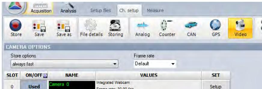
As always, be sure to press in as **USED** any of the video streams or cameras that you want to be able to display and record with your data files.
