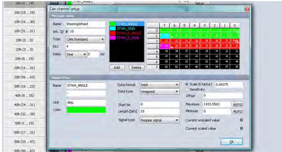
In the top half of this dialog you set up the message itself, where in the bottom half you can configure the channels contained within this message.
