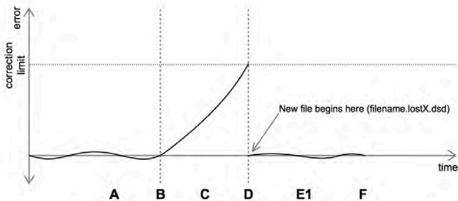
As soon the timing device is selected DEWESoft automatically sets the data acquisition hardware to external clocking for receiving the sample frequency out of the GPS-CLOCK. In addition to this each measurement starts synchronized with the PPS signal. The time information of the data file is taken out of the GPS-time and not anymore from the local PC time.
