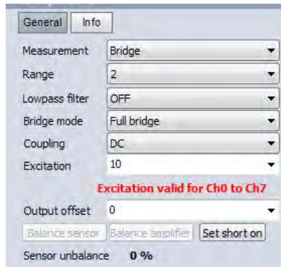
Select the full bridge mode of the MDAQ-SUB-BRIDGE, and then plug in the completion adapter.
