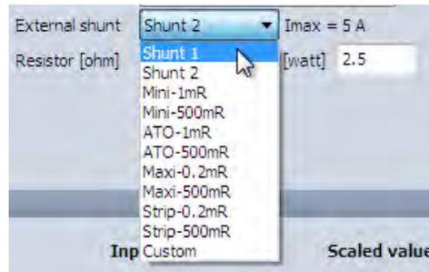
Simply select the shunt that is appropriate. In this case, when you choose Shunt 1, DEWESoft will automatically scale the input. And notice that the measuring ranges are now given directly in mA instead of voltage units.
