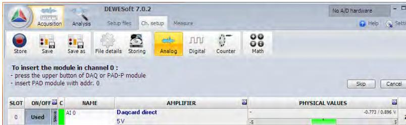
Follow the instruction to press the TOP black button on the module in the first slot, which is always SLOT 0 in the case of doing a FILL RACK, since you are starting at 0 and going all the way up, filling all modules.
