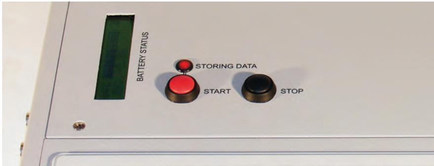
The built-in LED will illuminate when data is storing. When you press STOP, the LED will go dark, and the storing will stop.
