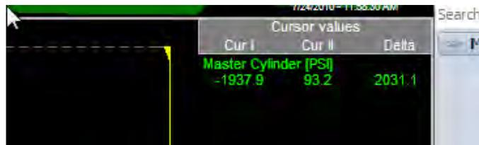
So we see the value of the channel called Master Cylinder at cursor I, cursor II, and then the calculated delta amplitude value.
