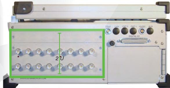
Note - if your system is ordered with any 1.5U MDAQ panel (MDAQ-SUB-V200-BNC or MDAQ-SUB-ACC-BNC are perfect examples), and you do not order a 0.5U accessory panel, we will install a blank panel in the 0.5U space.
