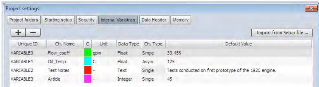
Above we have created four variables - one of each basic type: text, floating number, and integer number. In addition, there are two versions of floating numbers: one which is async and another which is a single value.
