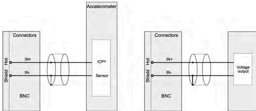
Above left: IEPE sensor mode    Above right: Voltage input mode
