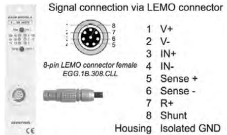
⇒ **CAUTION: The sensor shield can be connected to either pin 4 (SUB-D version only) or the housing of the 9-pin SUB-D / 8-pin LEMO connector, depending on your application.**
