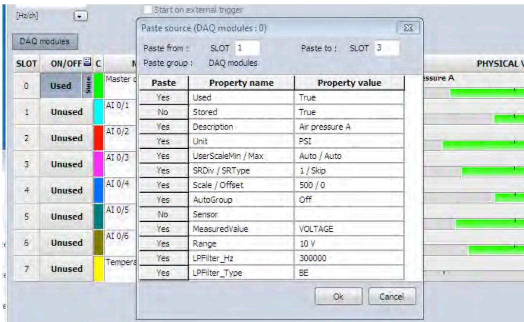
You can click the boxes in the PASTE column to toggle whether this parameter gets pasted or not. As mentioned, the Used/Unused status is not normally pasted from one channel to another, but here we can override that and paste that, too, as well as the channel name, etc. At the top we told it to paste from Slot 1 to Slot 3, so that channels 1, 2, and 3 will receive this paste simultaneously. Click OK to execute the paste, and see what happens:
