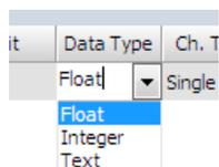
If it is a numeric type, you can set the channel type to single or async. This does not apply to text data types.
