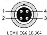
**xPAD2-V8 signal interface connector**
