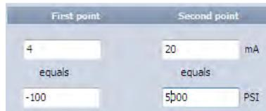
That's all you would have to do! Any scaling parameters which are linear can be entered in this way.
