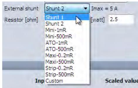
When you do this, the software allows you to enter the value of the shunt resistor that you are using, as well as the maximum wattage. The software will do the appropriate ohm's law calculations to amperage for you automatically.
