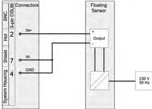
Current measurement, external shunt
