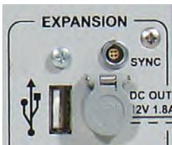
There are sync and USB 2.0 connectors located in the EXPANSION group. Connections to at least USB and SYNC are required required to connect a DEWE-43 expansion module.
