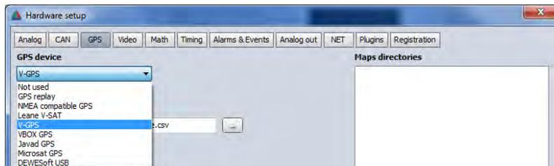
You will need to also configure the interface that these parameters are coming across. Typically this will be a COM port with a relatively high number. There is no harm in starting with the highest com port number and working your way down until you find the correct one. The screen will show all of the parameters available for setting when the GPS-CLOCK interface is correctly identified here.
