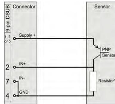
☺ **The value of the resistor depends on the sensor supply voltage and the open collector sensor.**
