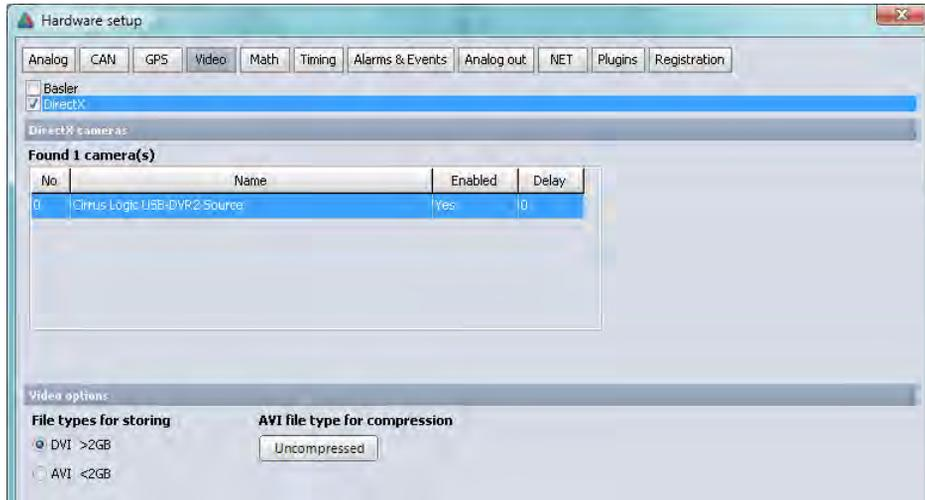
You need to enable **DIRECTX** video via the checkbox. When you do, the **VIDEO-FG4** card should show up automatically, and four video channels should appear in the list. If this does not happen, then the card is not set up properly under Windows, because DEWESoft will always see any properly configured DirectX video sources that are available under Windows.
