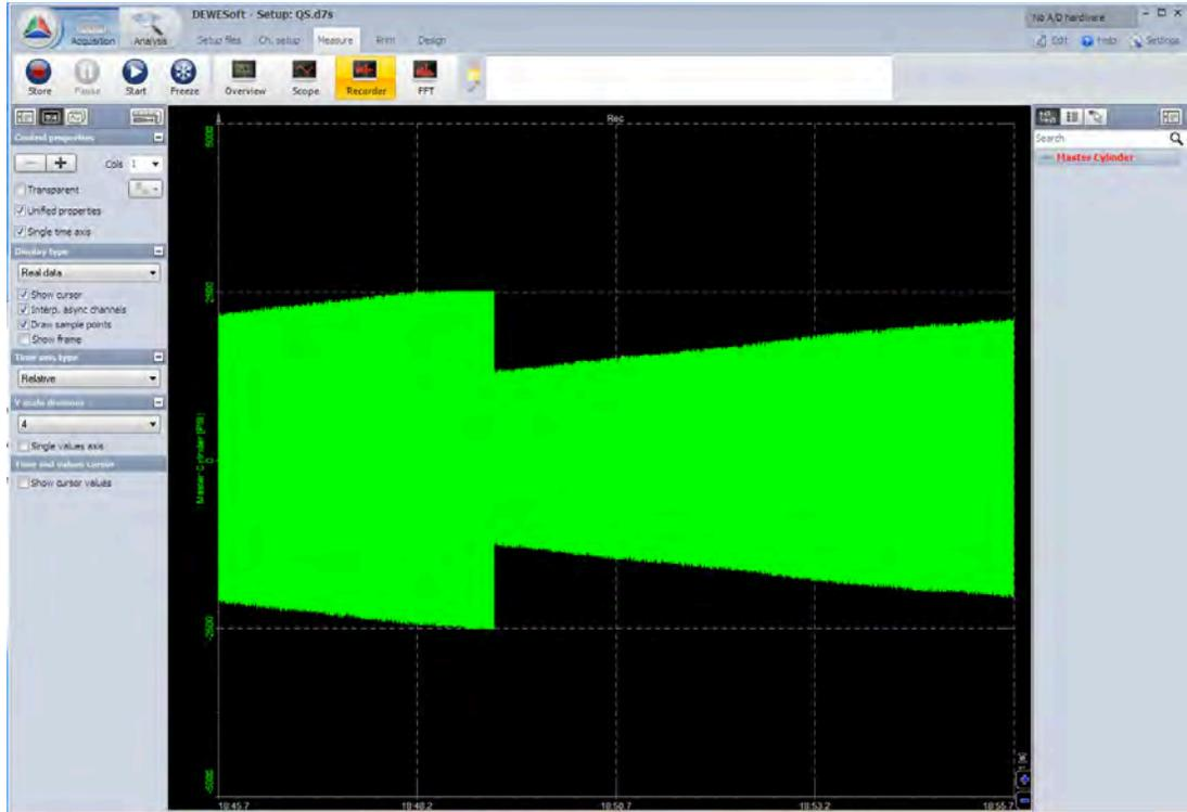
The recorder shows you one big graph by default. Or perhaps more graphs depending on how many channels were set to USED when you first come here after leaving the setup screen. We had only one channel USED, so DEWESoft gave us one graph with our one channel on it. Common questions at this point:
