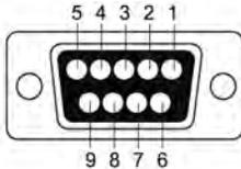
⇒ **CAUTION: The sensor shield can be connected to either pin 4 (SUB-D version only) or the housing of the 9-pin SUB-D / 8-pin LEMO connector, depending on your application.**
