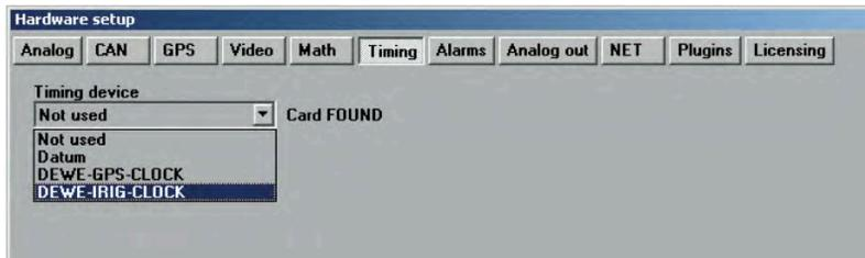
The interface should then be located and shown on this screen. When hardware is successfully found, you can select either IRIG A or IRIG B as Coding type and AC modulated or DC signal type:
