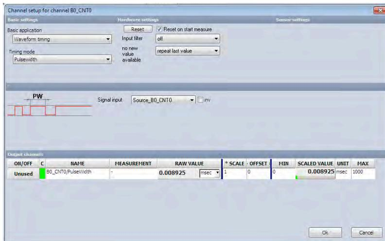
🕒 **Note:** to measure the LOW time of the signal, invert the input.
