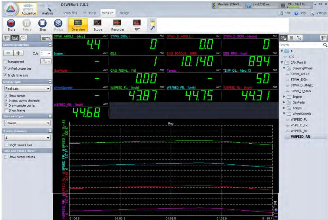
Notice that the CAN channels are shown on the right side of the screen in the CHANNEL LIST. A nice feature is that the channels contained within each message are collapsed into a group whose name is the same as the message name:
