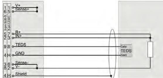
⇒ Sense leads (SUB-D: pin 3 and 6; LEMO: pin 5 and 6) MUST be connected!
