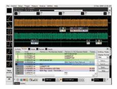
Trigger on and decode PCIe serial packets.
