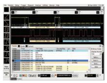
Trigger on and decode JTAG packets.
