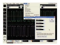
Ever wanted to change the scale or offset of a function or waveform memory? If you have, you know that it requires multiple menus and key strokes. In Infiniium software version 2.01 and later, you can now map functions and waveform memories to the front panel controls of the oscilloscope!
