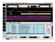
Trigger on and decode MIPI packets.
