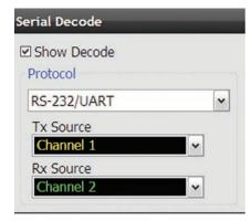
Trigger on and decode RS-232/UART transmission.
