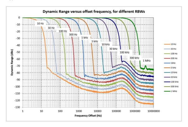
$<sup>^{\</sup>mathrm{1}}$  For 1 MHz RBW, the sideband observed may degrade the dynamic range to -70 dBc
