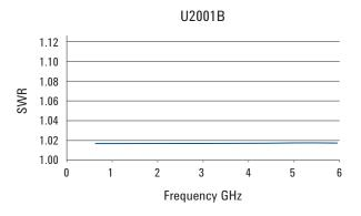
Typical SWR for U2001B sensor (25 °C ± 10 °C)
