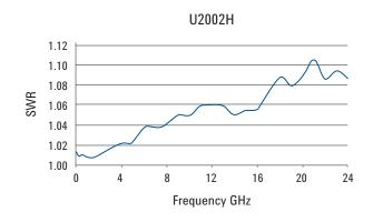
Typical SWR for U2002H sensor (25 °C ± 10 °C)
