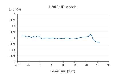
*Typical power accuracy at 25 °C for U2000/1B sensors*<sup>1</sup>
