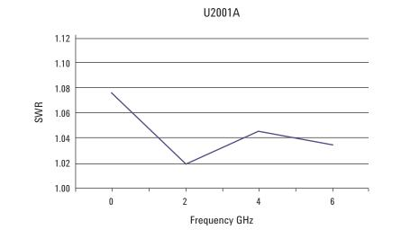
Typical SWR for U2001A sensor (25 °C ± 10 °C)
