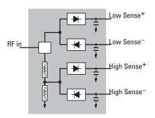
This technique ensures diodes in the selected signal path are kept in their square law region-with output current and voltage proportional to input power. The diode pair/attenuator/
