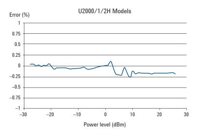
1. Measurement uncertainty ≤ 1.6%. At room temperature and excluding power level dependent terms (zero set, drift and noise)
