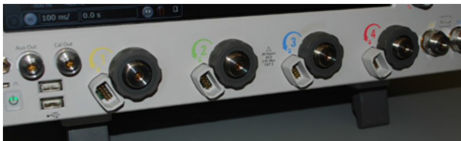
Figure 3 Z-Series oscilloscope probe connectors
