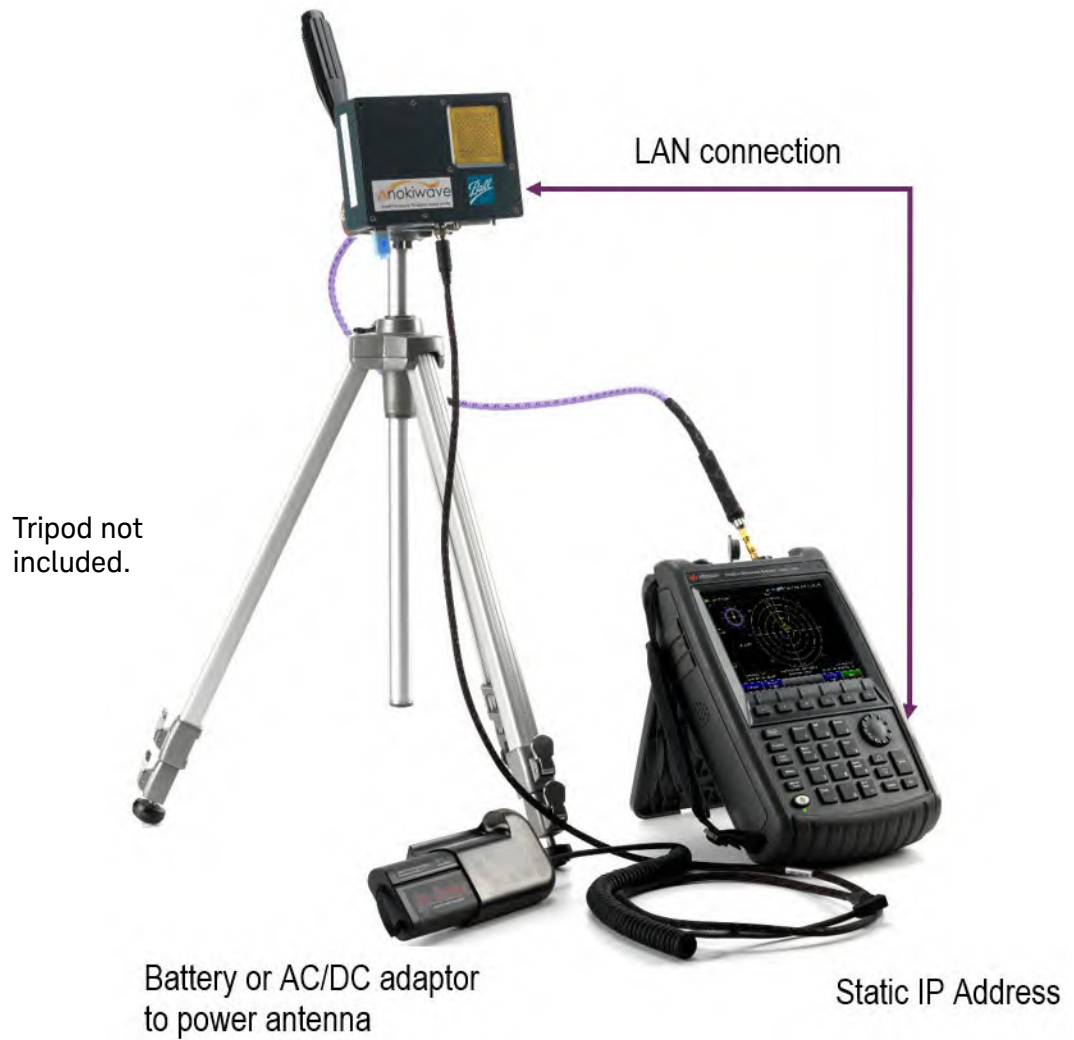
Figure 14-1 Example of local point-to-point LAN connection
