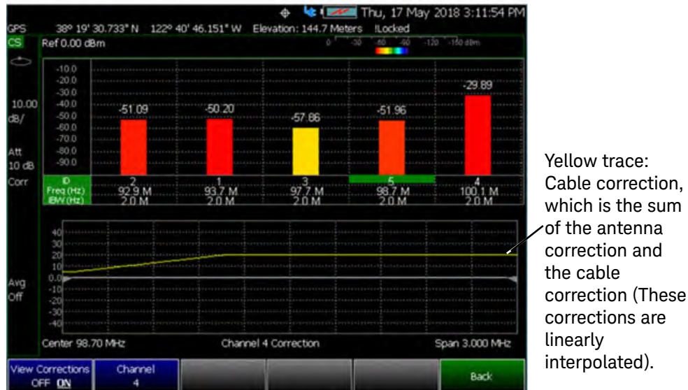
Figure 28-23 Yellow Trace with Cable and Antenna Corrections
